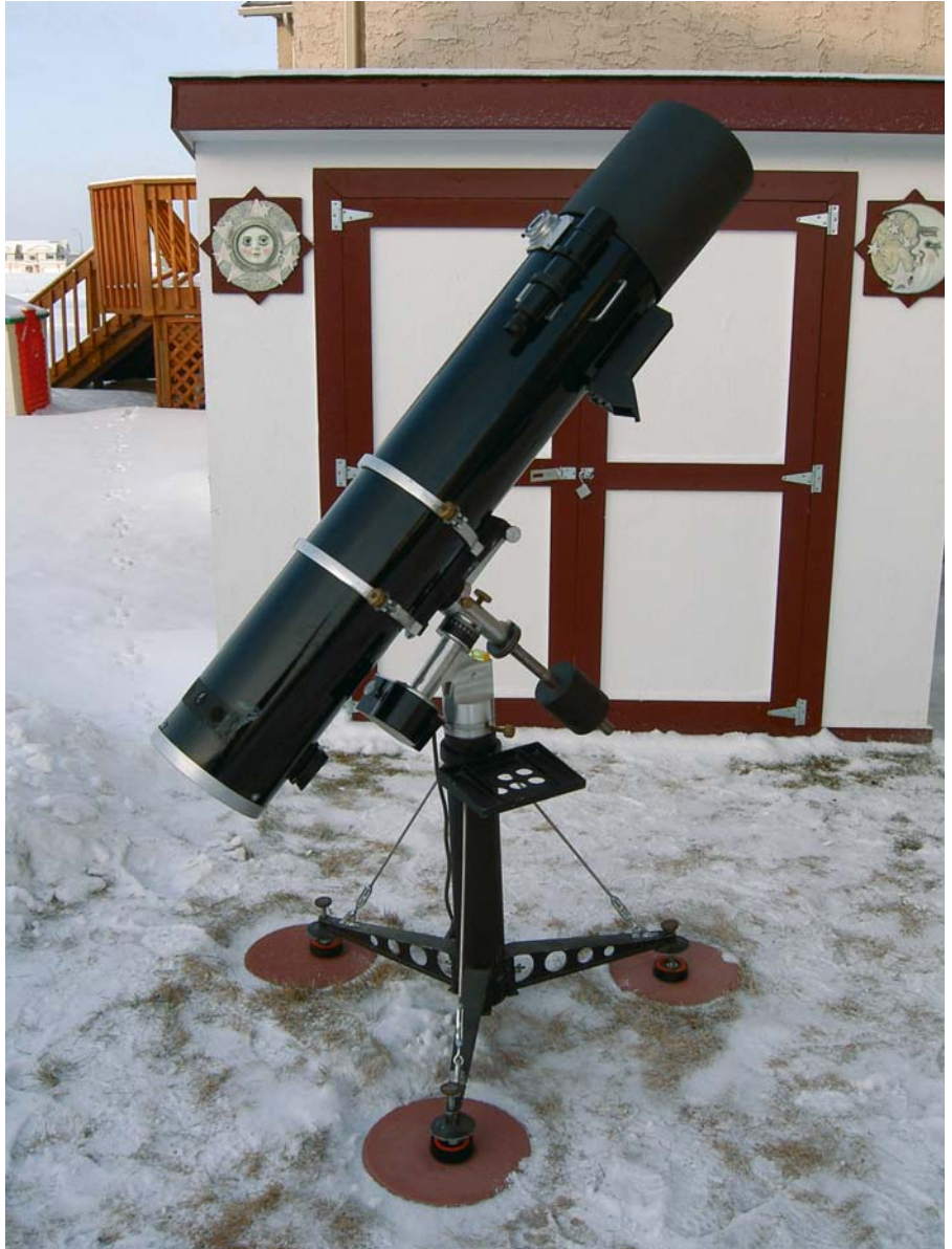
Figure 2.3. Newtonian reflectors, like this 20.3-cm (8.0-in) f/6 , are among the most popular telescope designs for observing the planets, especially in focal ratios f/6 or greater. (Credit: Mike Karakas, Winnipeg, Ontario, Canada; ALPO Saturn Section.)
