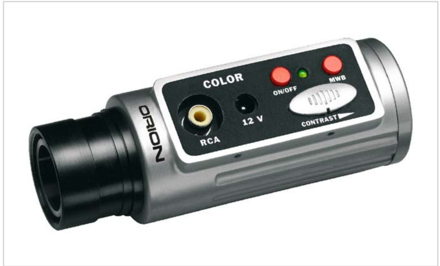
Figure 9.3. Available in color and monochrome models, battery-powered electronic imaging eyepieces, like the one shown here, neatly fit into the focusing tube of most telescopes and will transmit live video images of Saturn via a small RCA cable to a TV monitor for viewing or a VCR for recording. They contain CCD detectors like the chip in a video camcorder, and although they work fine for planets and the moon, they are not sensitive enough for imaging faint deep sky objects. (Credits: Orion Telescopes and Binoculars.)
