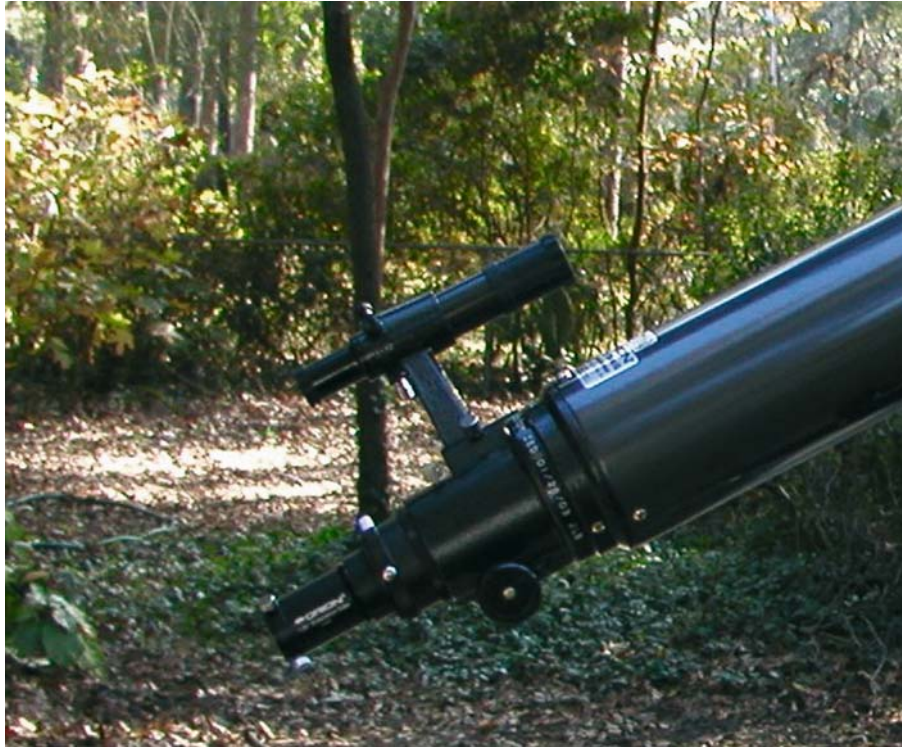
Figure 2.13. A small 6- × 30-mm finder, properly aligned along the optical axis of the main instrument, is sufficient for centering bright planets like Saturn in the telescope’s field of view. (Credit: Julius L. Benton, Jr.)
