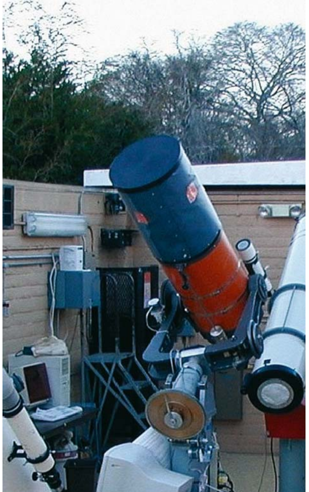
Figure 2.4. With focal ratios ranging from f/10 to f/15 , Cassegrains are often well suited for planetary work and are quite compact compared with Newtonians and long focus refractors. (Credit: Brian Cudnik, Houston Astronomical Society; ALPO Saturn Section.)
