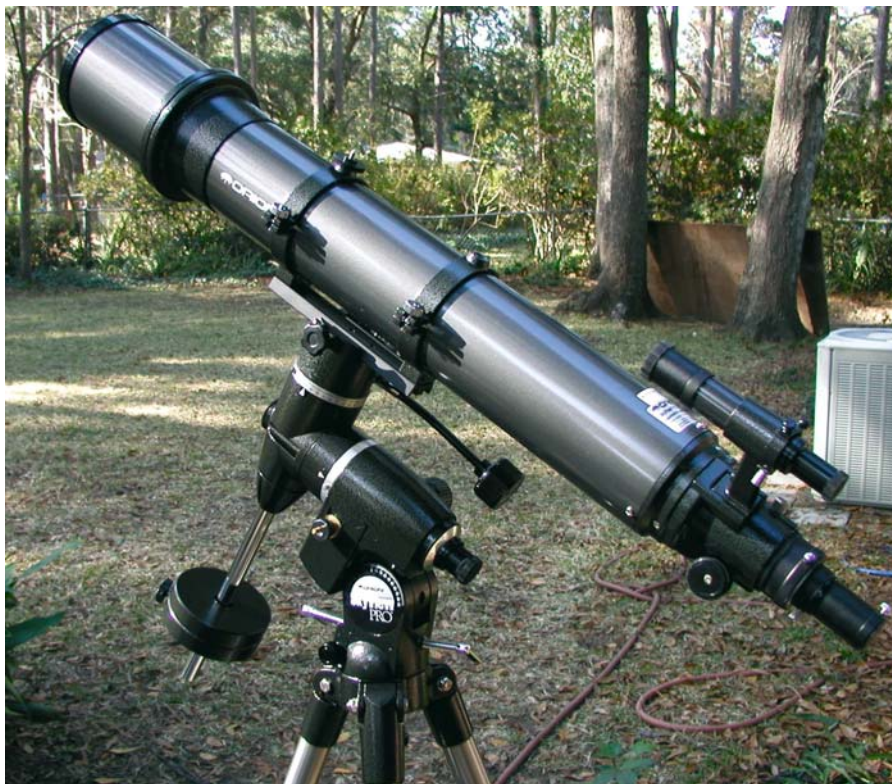
Figure 2.2. A modern 12.0-cm (4.7-in) achromatic refractor mounted on a sturdy equatorial mounting. Top-quality refractors may be the best all-round instruments for observing planets because of their sharp, high-contrast images. (Credit: Julius L. Benton, Jr.)
