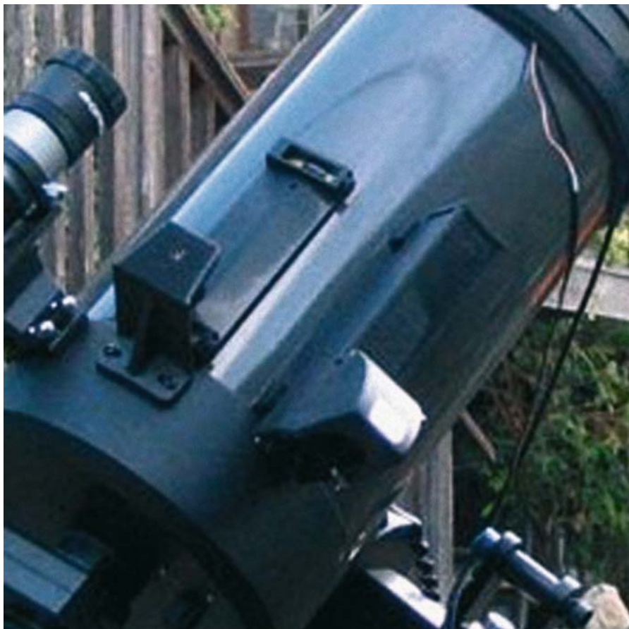
Figure 2.14. This small reflex sight is extremely effective in finding objects once its alignment is coincident with the main telescope. (Credit: Jason P. Hatton, Mill Valley, CA; ALPO Saturn Section.)
