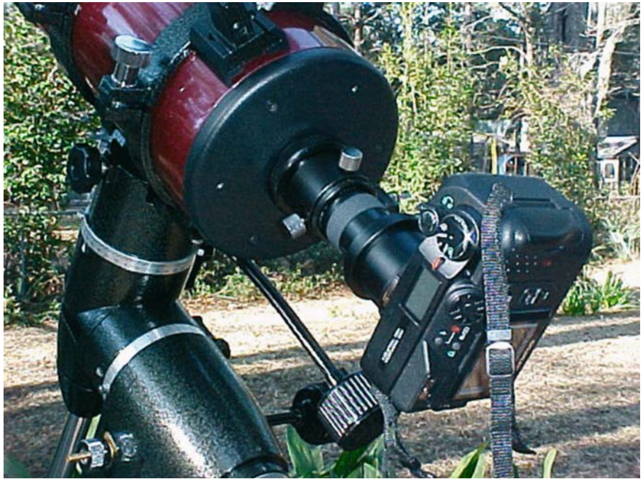
Figure 9.6. The author's high-resolution 4.1-megapixel digital camera, shown here, conveniently attaches to the focusing tube of the telescope using a special adapter that couples to both the eyepiece and lens housing of the camera. (Credit: Julius L. Benton, Jr.)
