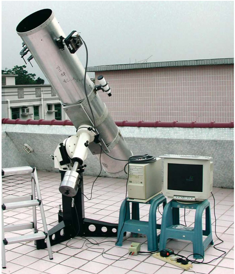
Figure 9.4. A very impressive CCD array coupled to a 31.8-cm (12.5-in) Newtonian owned by Eric Ng of Hong Kong. (Credit: Eric Ng; ALPO Saturn Section.)
