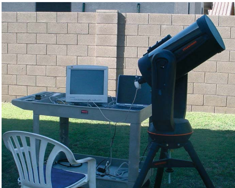
Figure 9.8. Paul Maxson of Phoenix, Arizona, uses this 23.5-cm (9.25-in) SCT and webcam setup to regularly image Saturn and other solar system objects. (Credit: Paul Maxson; ALPO Saturn Section.)
