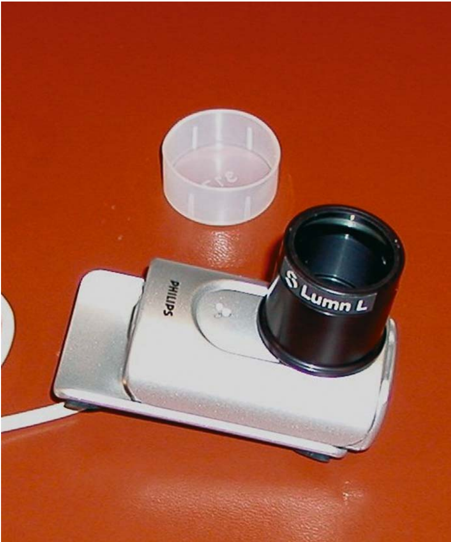
Figure 9.7. The author's webcam pictured here is extremely lightweight, connects to a laptop computer via a USB cable, and comes with an adapter that slips into the drawtube of a telescope's focusing mechanism. An IR blocking filter, which is highly recommended (see text), threads easily onto the webcam. (Credit: Julius L. Benton, Jr.)
