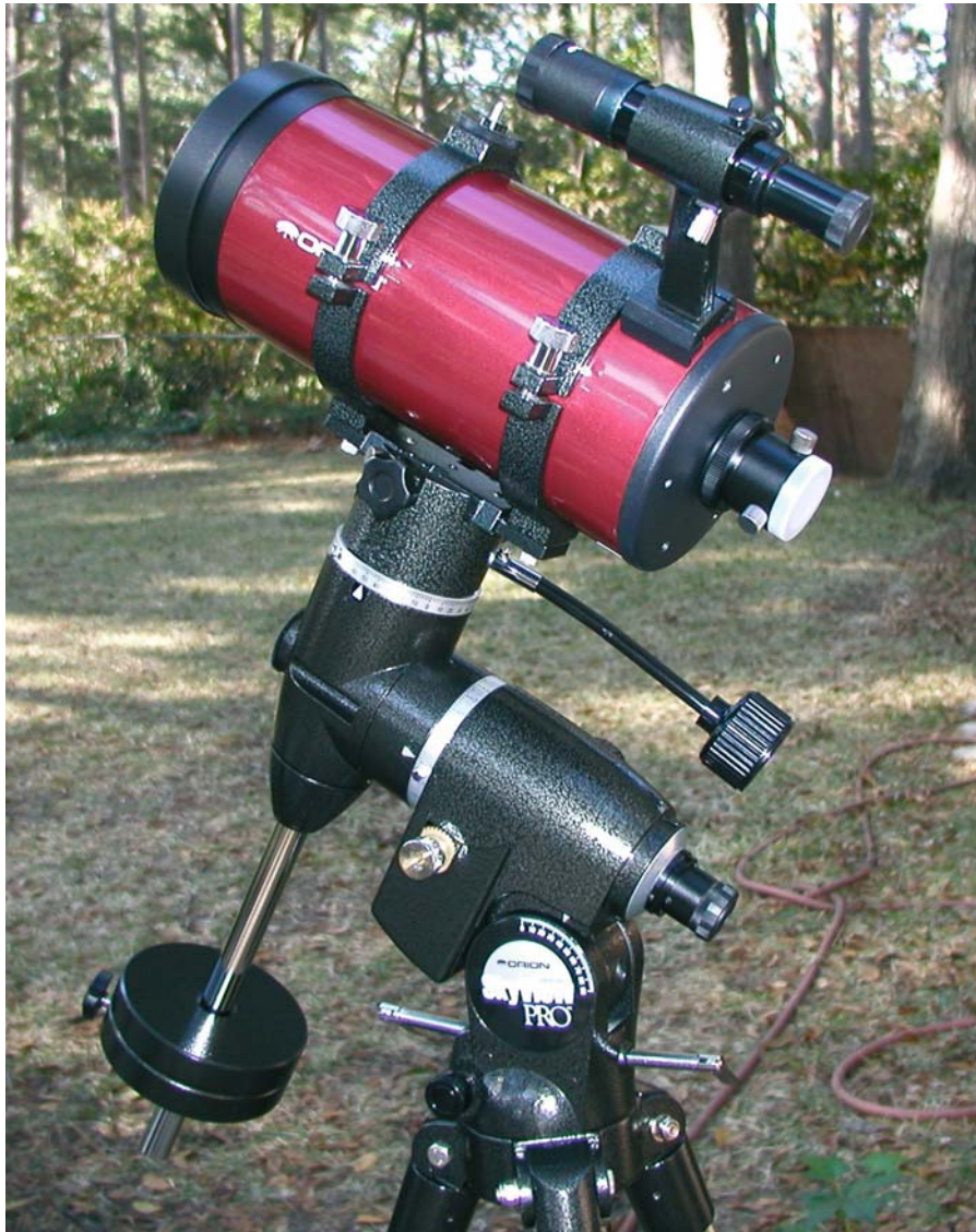
Figure 2.7. A sturdy conventional German equatorial mounting with field tripod, slow-motion controls, and a battery-powered clock drive supporting the author's highly portable 12.7-cm (5.0-in) f/13 Maksutov-Cassegrain. (Credit: Julius L. Benton, Jr.)
