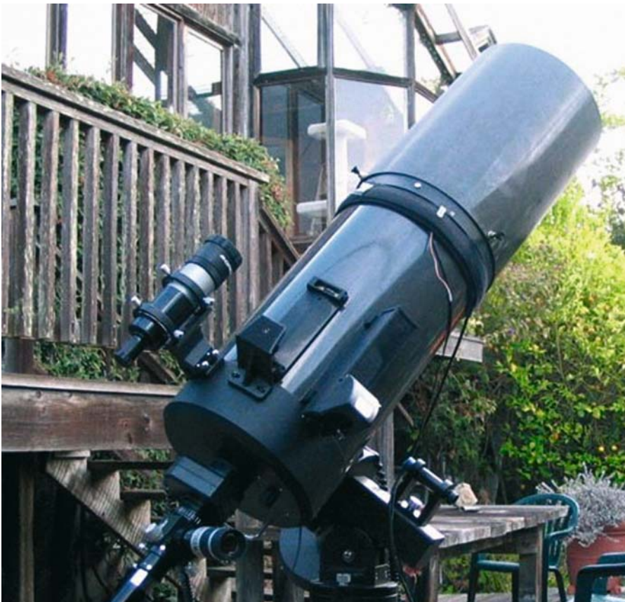
Figure 2.5. A well-equipped 23.5-cm (9.25-in) Schmidt–Cassegrain telescope. Although compact, it is near the upper limit for transport into the field for observing. The SCTs often perform well in viewing planets like Saturn as long as their collimation is correct. (Credit: Jason P. Hatton, Mill Valley, CA; ALPO Saturn Section.)
