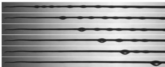
*Figure 10.* Successive snapshots (interval between each picture: 10 s) showing the evolution of a liquid film (thickness between 8 and 25  $\mu\text{m}$ ) made of silicone oil ( $\eta = 20$  mPa.s and  $\gamma = 20$  mN/m) deposited on a conical fiber (of radius between 100 and 300  $\mu\text{m}$ ). (Reprinted with permission from [16]. Copyright Cambridge University Press.)
