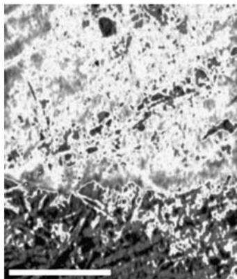
*Figure 14.* A section through the mid-plane of a paper sheet using X-ray tomography. Again the liquid, flowing from top to bottom, has been snap-frozen during wetting and is seen in light grey, with voids as dark to black. Note the voids shown do not connect with either surface of the sheet and represent trapped air. Scale bar = 350 microns.
