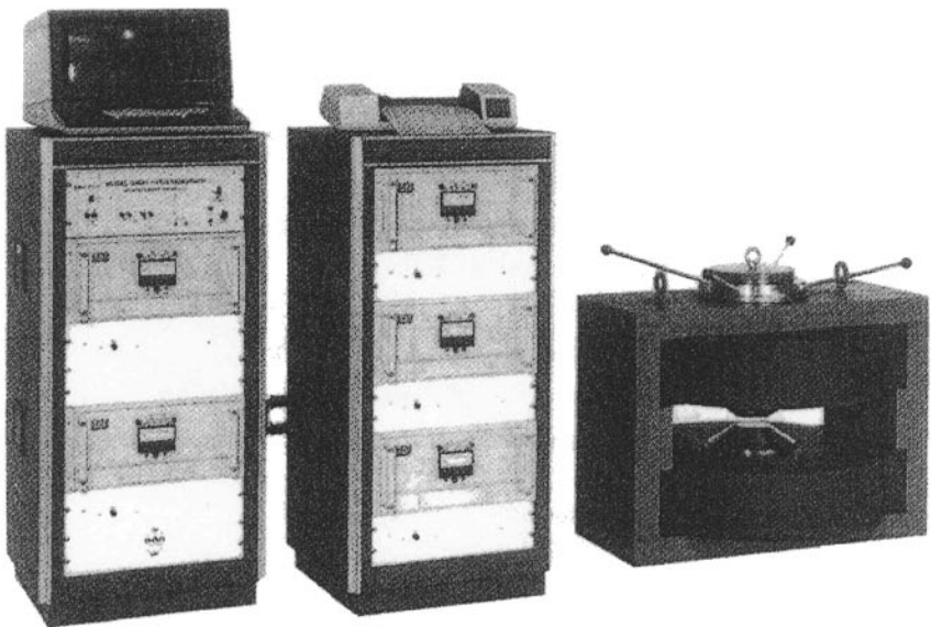
Figure 18.5- B-H Plotter for hard and soft magnetic materials, Photo, Courtesy of I.D.J Inc. , Troy, Michigan.
