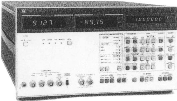
Figure 18.10- Hewlett-Packard impedance analyzer, from Hewlett-Packard Test and Measurement Catalog(1989) Hewlett-Packard Co.,Palo Alto, CA
