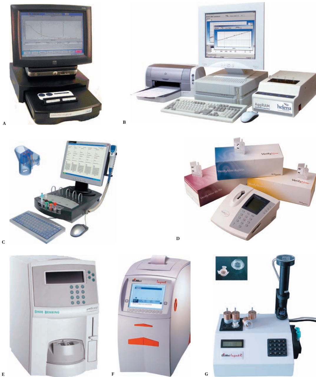
Figure 22.1 (A) An example of a modern eight-channel platelet aggregometer. The model shown is the Biodata PAP-8E (reproduced with permission from Biodata). (B) An example of a modern four-channel modular platelet aggregometer. Additional four-channel modules can be added into the system depending upon workload demand. The model shown is the Helena AggRAM system (reproduced with permission from Helena Biosciences). (C) The Multiplate ® multiple platelet function five-channel impedance analyzer. The inset illustrates the disposable cuvettes with electrodes (reproduced with permission from Hart Biologicals). (D) The VerifyNow ® assay, previously known as the Ultegra Rapid Platelet Function Analyzer (RPFA). The three types of cartridge systems available are shown in the background: the VerifyNow ® IIb/IIIa, VerifyNow ® Aspirin, and VerifyNow ® P2Y12 (reproduced with permission from Accumetrics). (E) The PFA-100 ® instrument (reproduced with permission from Dade-Behring). (F) The Diamed IMPACT ® device (reproduced with permission from Diamed). (G) The Diamed IMPACT-R ® device (reproduced with permission from Diamed). The cone and plate are shown in the inset.
