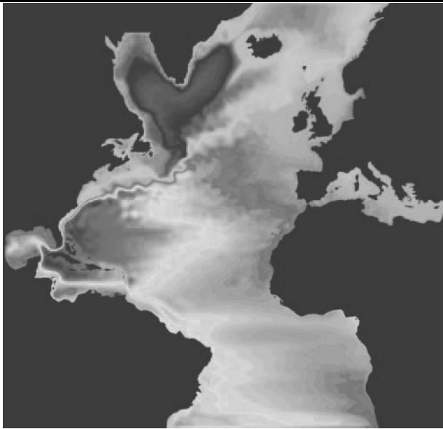
Figure 5.54. (in color on page 520). Plot of the two-year mean of the sea-surface height of a high-resolution ( 1/12^\circ ) simulation with MICOM (Chassignet and Garaffo, 2001).
