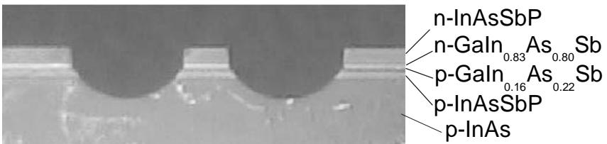
Figure 11. Etched profile of double-channel stripe laser structure
