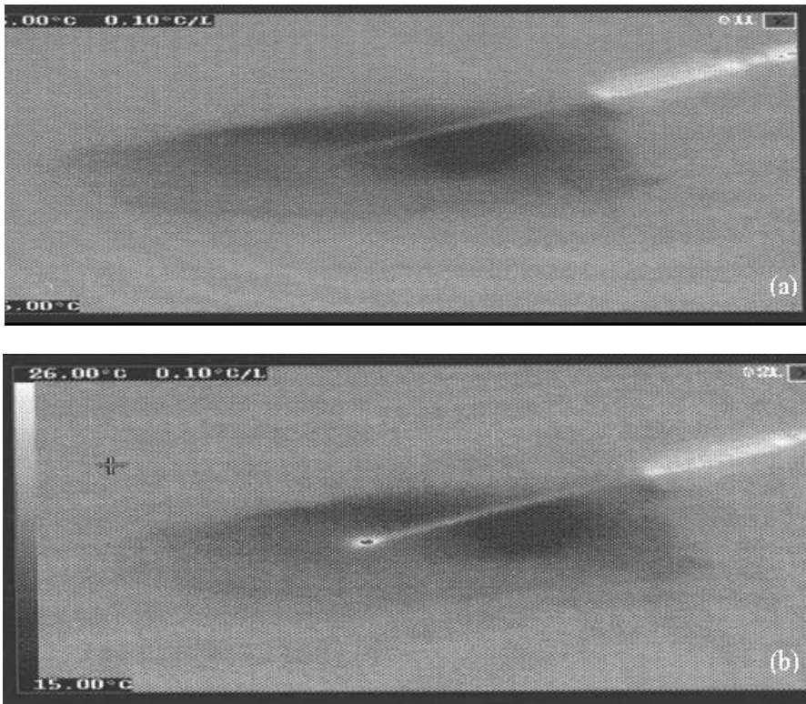
Figure 9. Typical thermal images obtained using mid-IR laser irradiation (see Figure 7) of chicken skin after 10 laser pulses when the OF tip is above the skin surface (a) and after a single laser shot when the smart tip is on the surface (b)
