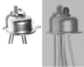
Figure 20. Photos of the LEDs with chalcogenide ( right ) and sapphire ( left ) lenses mounted onto a TO-18 header
