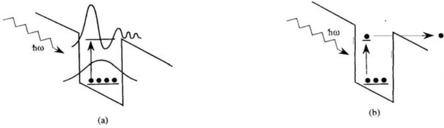
Figure 1. Conduction band profile of a bound-to-bound transition: (a) a photon having energy h\omega excites an electron in the ground state to the excited state and (b) the photoexcited electron tunnels out of the well and thus contributes to the photocurrent
