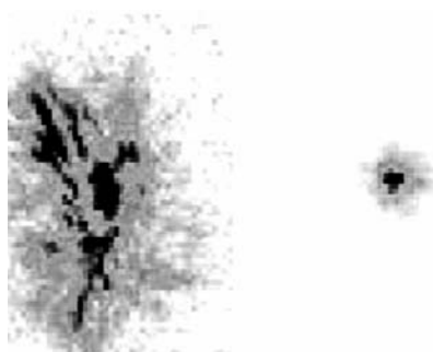
Figure 5. Atmospheric turbulence effects ( left ) and the corrected beam ( right )
