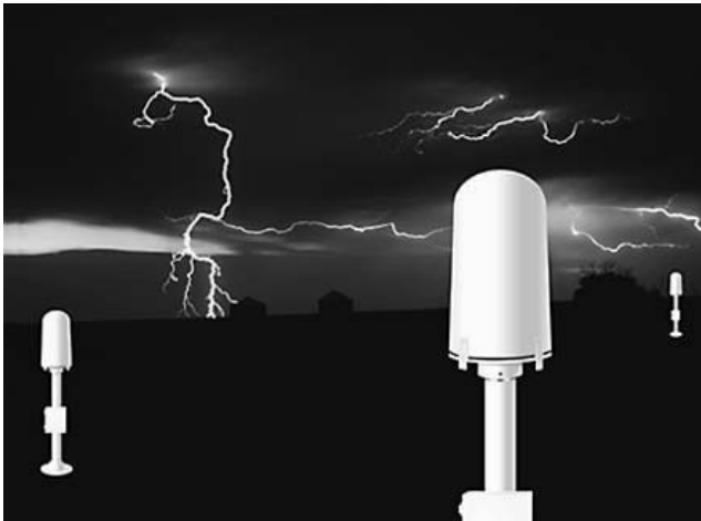
Fig. 4.2. Lightning detectors installed by the Meteorological Institute in Portugal
