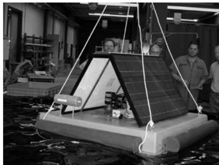
Figure 7. This is a BGR-instrumentation equipped to monitor gas flux and gas composition on mud volcano lakes.
