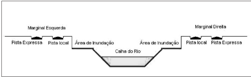
Fig. 14-4. Channel of the Tietê River working with a normal regime
