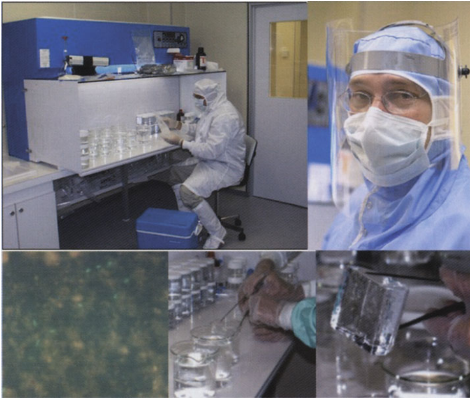
Fig. 7.17. View of the clean room lab, operator protection and some handling and washing operations used in ice core decontamination at LGGE in Grenoble. Bottom left: A microphotograph view of contamination of an accreted ice sample by the drilling fluid. Due to the small size of the ice sample, application of the full decontamination process was not possible. Once filtered and coloured by DIAPI, sediment inclusions (clays mineral) appear in yellow while microorganisms (such as cocci) appear in fluorescent green.
