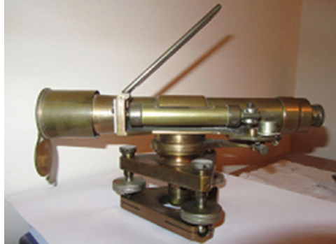
An original three screw dumpy level
