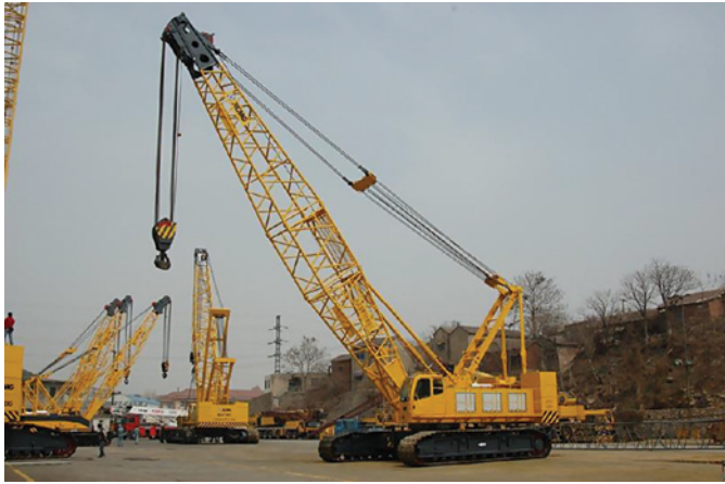
Large tracked crane with lattice jib used for heavy lifting operations
