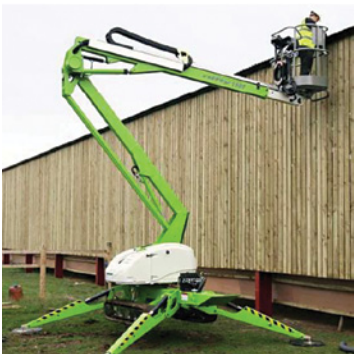
Track mounted lifter with stabilisers
