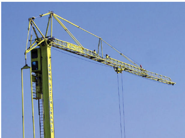
Self-erecting tower crane with horizontal jib (horizontal jib tower cranes are also available)
