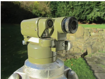
A ball and socket quickset level – a Swiss-made Kern instrument
