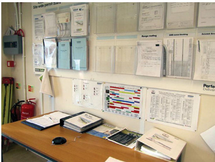
Permit board where site personnel can collect daily permits. Display area showing site photographs file and visitors' information.
