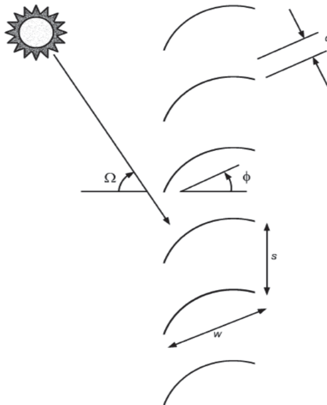
Figure 3.1 Geometry of Slat-Type Sunshades
