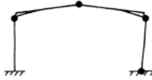
Figure 11.11 Basic collapse mechanism (Mode 1) for haunched portal.
