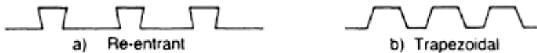
Figure 9.13 Typical profiles-various depths, various forms of indentation and various types of stiffening are used.
