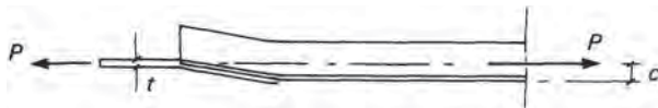
Figure 3.7 Bending of gusset to permit reorientation of load in angle connected to one leg.
