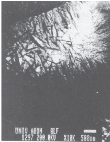
Figure 3.4. Scanning Transmission Electron Microscopy micrograph of a well-crystallized hydrotalcite-like phase which has developed within the original contours of a fully hydrated slag particle (ISH). [11]
