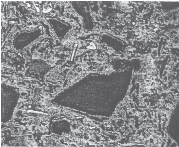
Figure 3.3. Backscattered image of a reacted zone enveloping a slag in blast furnace cement hydrated for 90 days. [11]
