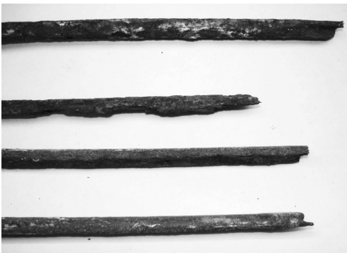
Figure 7. Profile of corroded strands.
