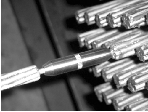
Figure 4. Exchange of a single strand in a test.
