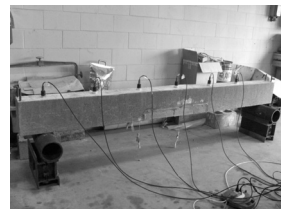
Figure 4. Accelerometric sensors location on the cracked and corroded beam.
