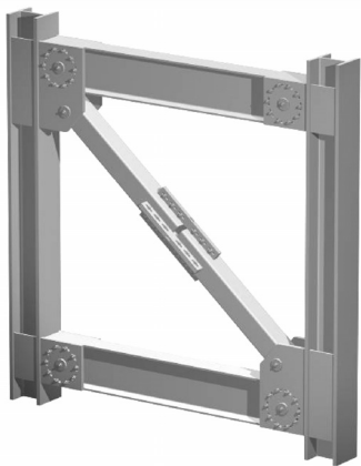
Figure 23. The pin-fuse frame, US Patent Pending.
