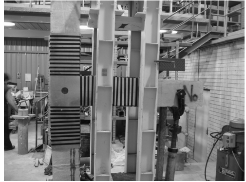
Figure 5. T-connection completed with steel straps.
