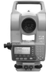
Figure 3. The developed light-wave survey camera with a built-in crack scale.
