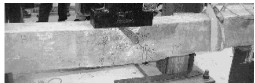
Figure 1. Beam (B1) after testing—1st set.
