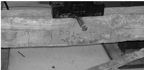
Figure 4. Debonding of CFRP in Beam (B6).
