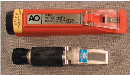
Figure 3-9 Hand held refractometers can be easily used to determine total plasma protein as well as urine specific gravity.
