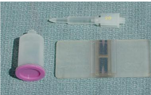
Figure 3-11 Unopette® diluting pipette and reservoir for counting WBCs and platelets in a hemocytometer.
