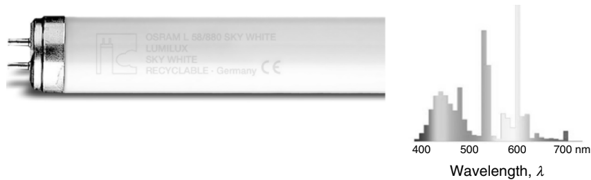
Fig. 1.16. Fluorescent lamp (FL): 58 W, \eta = 84 \text{ lm W}^{-1} , CCT 8,000 K, CRI >80, 1,500 mm overall length [133]
