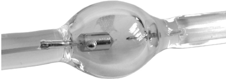
Fig. 3.21. Specially built dc high-pressure mercury discharge lamp for the investigation of the electrode temperature and the general electrode behavior at different electrode gaps, mercury pressures, electrode geometries, and lamp currents [8, 9, 11, 128]
