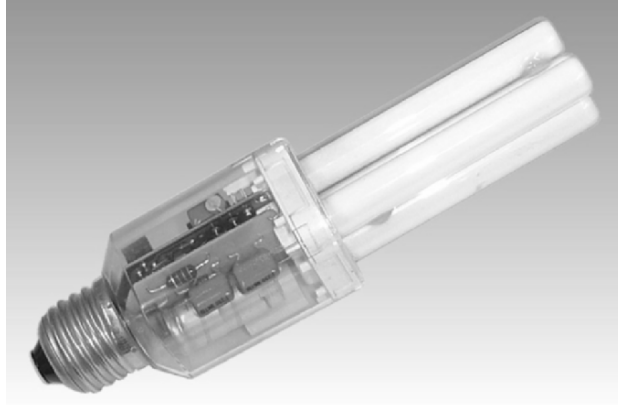
Fig. 1.18. Compact fluorescent lamp (CFL): 7 W, \eta = 57 \text{ lm W}^{-1} , CCT 2,700 K, CRI 82, 161 mm overall length [92]
