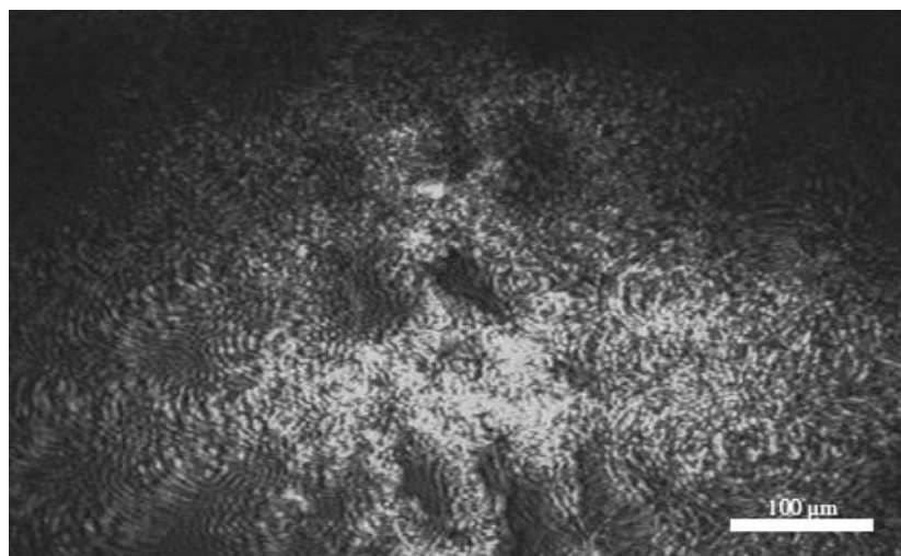
Fig. 1 Thin film of \text{CaCO}_3 below a stearic acid monolayer ( \Gamma_0 = 25 \text{ mN m}^{-1} , T = 22 \text{ }^\circ\text{C} , \text{pH} = 7 )
