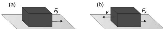
Fig. 3 a The friction force needed to initiate sliding from rest is known as the static friction force, denoted by F_s . b The force needed to maintain smooth sliding is referred to as the kinetic or dynamic friction force, denoted by F_k or F_f . v stands for velocity
