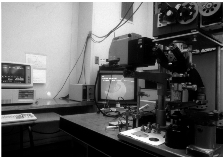
Fig. 1.35 This photograph shows the microscope, mounted DAC, echelle grating, video camera, computer with monitor and television with sample image and relevant data displayed on the screen [42]
