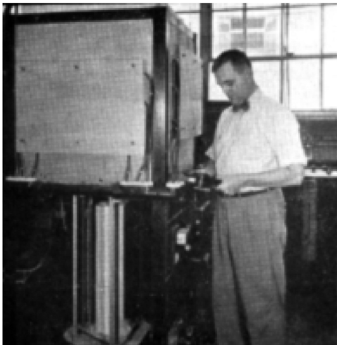
Fig. 1.3 Van Valkenburg (ca 1957) adjusting the parameters on his high-temperature furnace used for the synthesis, crystallization and reconstitution of mica [W. P. Richardson, NIST Photo Lab]
