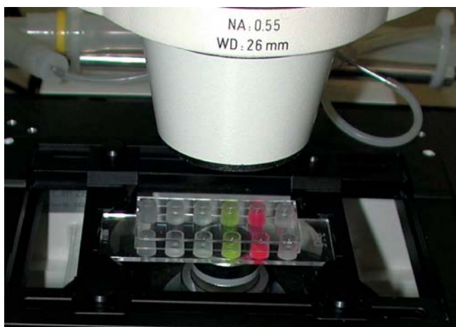
Fig. 5 Solutions of fluorescence standard dyes within the 30 \mu\text{l} channels of a microchannel microscopy slide ( \mu -Slide; ibidi GmbH, Germany)
