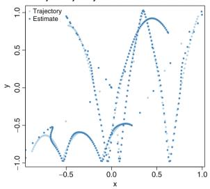
Fig. 10.1 Object trajectory and Kalman filter estimate
