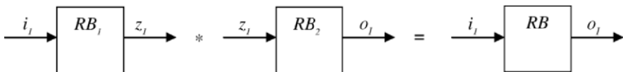
Fig. 5.3. Horizontal merging of rule bases RB_1 and RB_2 into rule base RB
