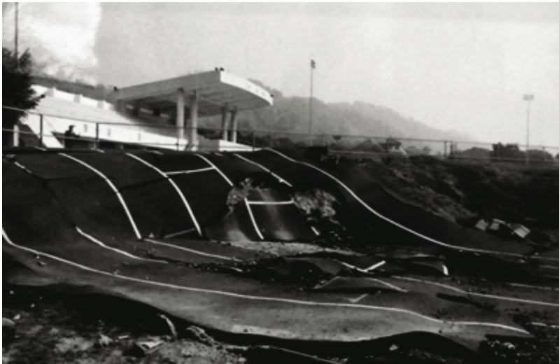
Fig. 1.4 Top panel: the bridge damage and scarp of 8 m height formed along the fault of the Chi-Chi earthquake on the river floor. Bottom panel: the fault scarp passing across the racetrack of one of the schools in Puli, Taiwan
