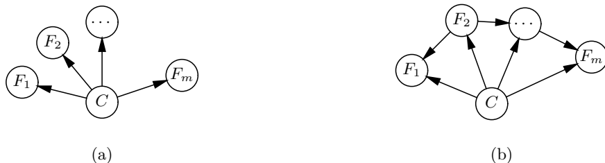
Fig. 2. A naive Bayesian network, (a), and a tree-augmented Bayesian network, (b); the nodes F_j indicate the feature variables and C is the class variable.
