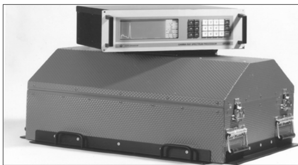
Figure 11.10. Gamma-ray spectrometer with a thallium-activated sodium iodide detector (photograph courtesy of Exploranium)
