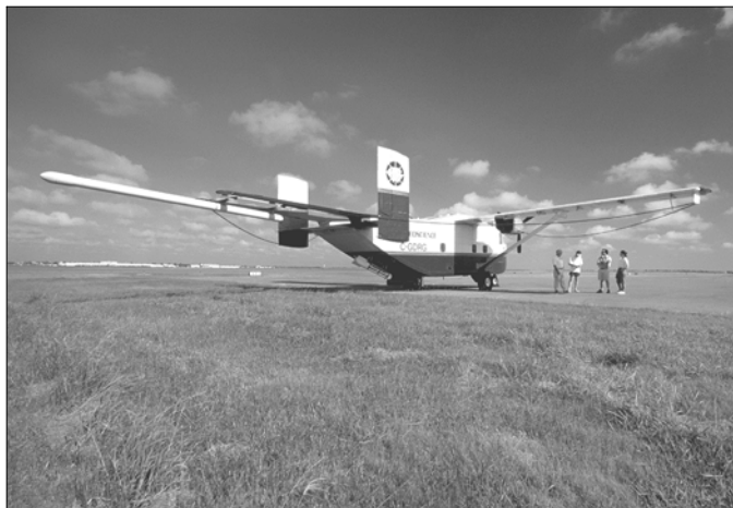
Figure 11.13. Survey aircraft carrying a stinger-mounted cesium magnetometer. Photograph by David M. Stephens.
