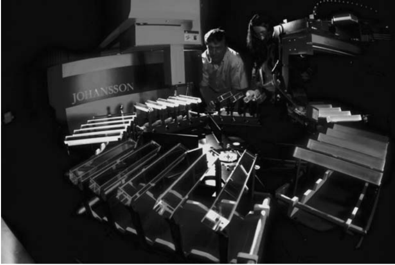
Fig. 6.2. Some of the 80,000 CMS crystals on the automatic certification device
