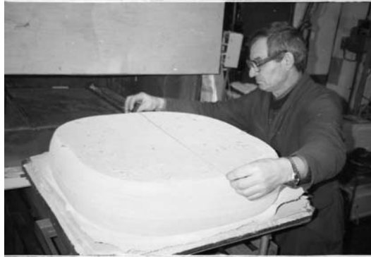
Fig. 4.2. A NaI(Tl) large size slab after press forging
