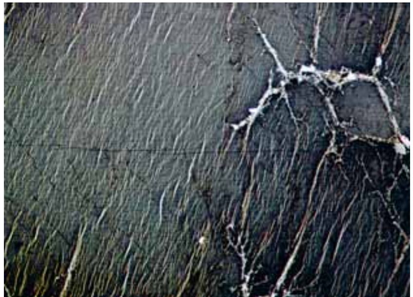
Figure 6.11 Photomicrograph of an alkali feldspar exsolution (magnification \times 40 ). Dark areas are orthoclase, light areas are albite. Each phase is homogeneous. (Mackenzie and Guilford, 1980)
