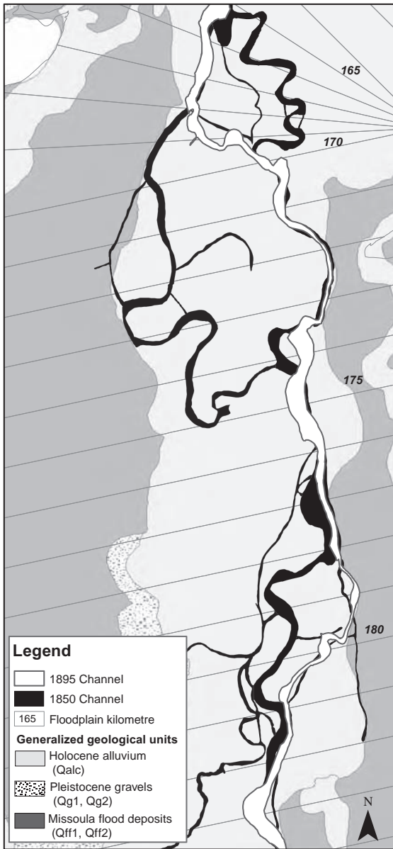
Figure 23.9 Example of avulsions 1850–1895 along upper Willamette River. Similar large-scale avulsions occurred along the entire Willamette River during this time period. In many cases, the 1895 channel avulsed into former side channels (e.g. FPKM 165–170) or carved cut-off channels (e.g. FPKM 169). (Geological map from O'Connor et al. , 2001. Historical Willamette River channel maps and floodplain transect maps from Hulse et al. , 2002)
