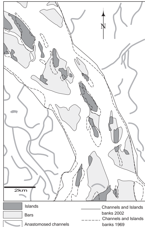
Figure 11.8 Recession of riverbanks by thermal erosion between 1969 and 2002 along the Lena at the latitude of Yakutsk city
