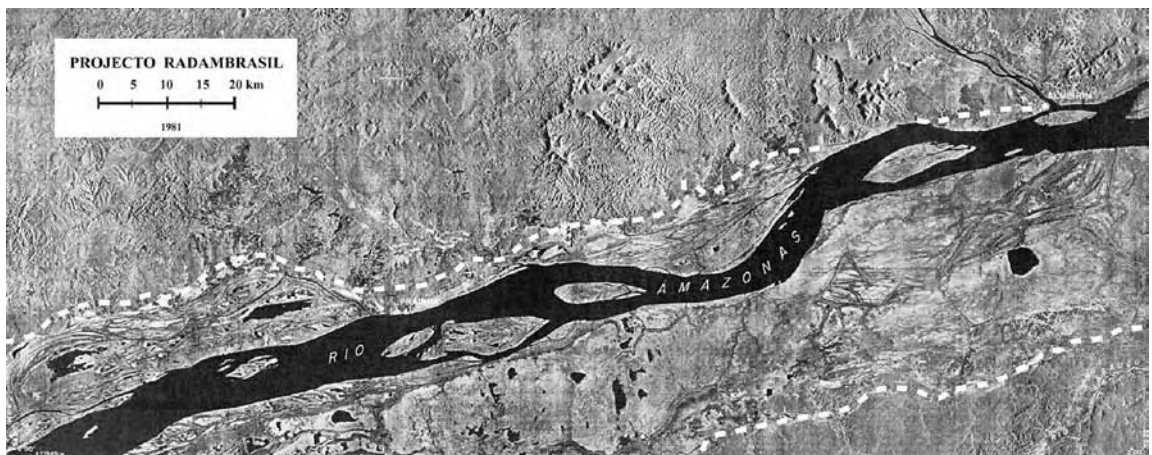
Figure 8.12 The Amazon River reach centred at 53^{\circ}15'W approximately at 3050 km on Figure 8.6b. Downstream of the Monte Alegre Intrusion the river is constructing a delta plain (between the dashed white curves) with rapidly shifting mid-channel bars and a floodplain that contains very few lakes. The absence of strongly developed scroll bars at the surface suggests intensive overbank sedimentation. Source: radar image from the Radambrasil Project
