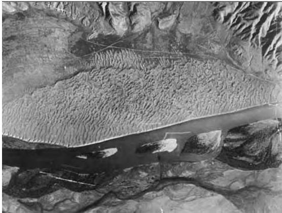
Figure 5.1 Aerial photograph of giant current ripples (gravel dunes) located near Kyzyl, Tuva. The ripples occur on a gravel bar just north of the Yenisei River (bottom of photograph) about 25 km southwest of Kyzyl. There are nearly 100 ripples on a bar 6 km in length. Ripple heights vary from 2 to 3 m. The photograph shows an area 6 \times 4 km. The palaeoflood flow was moving from right (east) to left (west)
