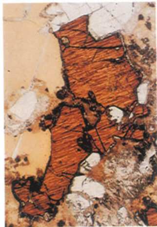
Figure 2.16. Coarse-grained priderite from the Walgidee Hills pluton, West Kimberley. Note the characteristic striped appearance. Field of view 1.6 mm.
