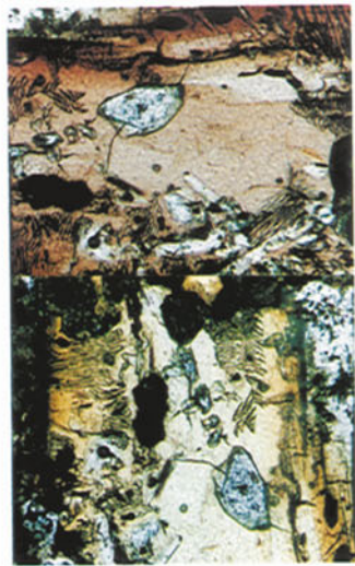
Figure 2.15. Characteristic reddish brown-to-yellow pleochroism of titanite and potassium richterite. This composite photomicrograph illustrates the appearance of a strongly zoned poikilitic plate of amphibole from Mt. North, West Kimberley in two orientations. Note the characteristic "fingerlike" fluid inclusions. Field of view 1.5 mm.
