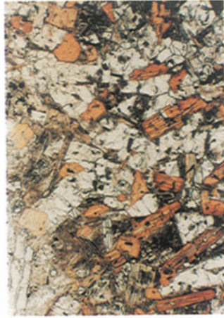
Figure 2.27. Phlogopite sanidine lamproite, Smoky Butte, Montana. Euhedral laths of zoned titanite phlogopite enclosed by subhedral prisms of sanidine (colorless). Interstices between the sanidine prisms are filled by brown titanite potassium richterite and/or glass. Opaque phase is armalcolite. Field of view 1.6 mm.
