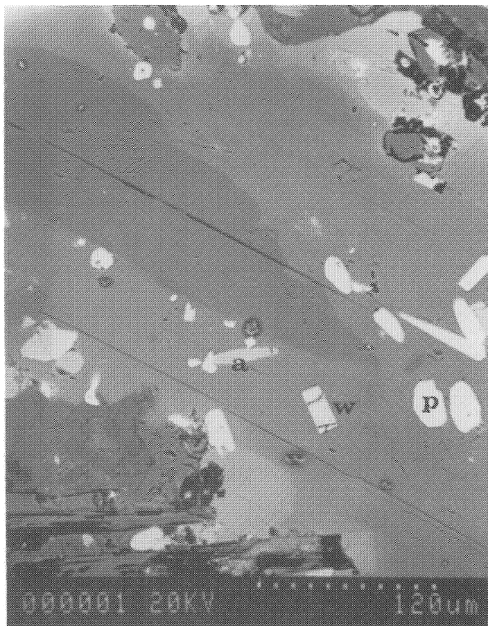
Figure 6.62. Characteristic morphology of euhedral wadeite (W), Mount North (West Kimberley). Also illustrated are priderite (P) and apatite (A). Backscattered electron image.
