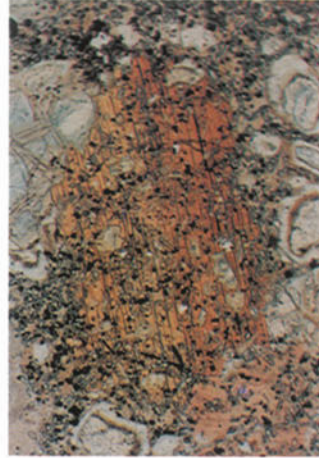
Figure 2.21. Groundmass poikilitic or madupitic titanian phlogopite. Madupitic olivine lamproite, Prairie Creek, Arkansas. Colorless prismatic crystals are diopside. Opaque euhedral crystals are spinel and perovskite. Field of view 1.6 mm.
