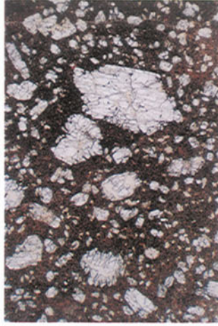
Figure 2.19. Olivine lamproite, Kimberlite Mine, Arkansas. Note the presence of resorbed macrocrysts of "dog-tooth" olivine (colorless) with serrate margins together with smaller euhedral-to-subhedral phenocryst olivines. The unresolved groundmass is rich in phlogopite, pyroxene, spinel, and perovskite. Field of view 10 mm.
