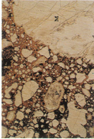
Figure 2.31. Hyalo-olivine lamproite lapilli tuff, Prairie Creek, Arkansas. Portion of a lapillus containing an olivine macrocryst (M) and a primary phenocrystal olivine (P) set in a light brown vesicular glass. Field of view 1.6 mm.
