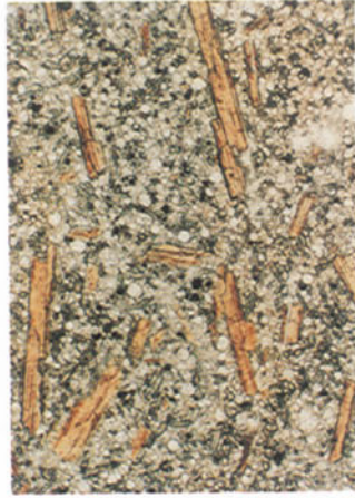
Figure 2.25. Leucite phlogopite lamproite, Emmons Mesa, Leucite Hills, Wyoming. Phenocrysts of microresorbed titanite phlogopite set in matrix of microphenocryst colorless rounded leucite crystals. Also present are small prismatic crystals of diopside (colorless). Field of view 1.6 mm.
