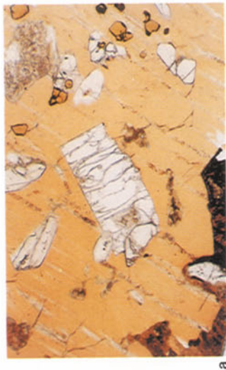
Figure 2.17. Characteristic appearance and habit of wadeite (a) in plane polarized light and (b) with crossed polars. The wadeite is enclosed by phlogopite and is associated with diopside (colorless and twinned), perovskite (deep yellow
