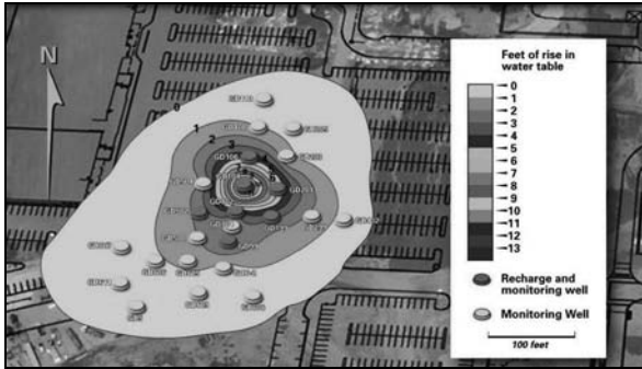
Figure 3. Measured water table mound during multi-well potable water injection
