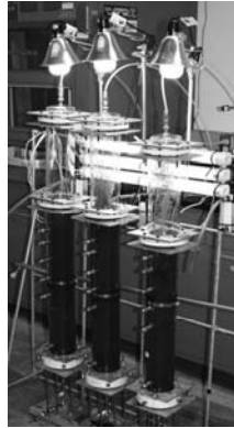
Figure 5. Laboratory bioretention columns (photo: LeFevre).
