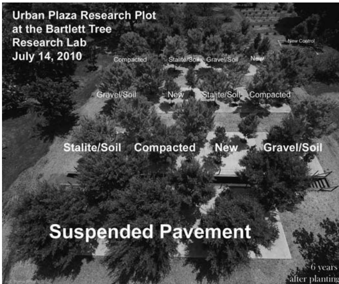
Figure 5. Comparison of trees grown in suspended pavement, compacted soil, stalite/soil, and gravel/soil 6 years after planting (Image courtesy of Thomas Smiley).
