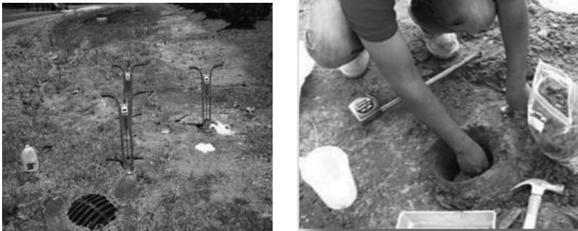
Figure 1. Double ring infiltration measurement installations and in-situ soil density measurement at Shelby Park biofilter.
