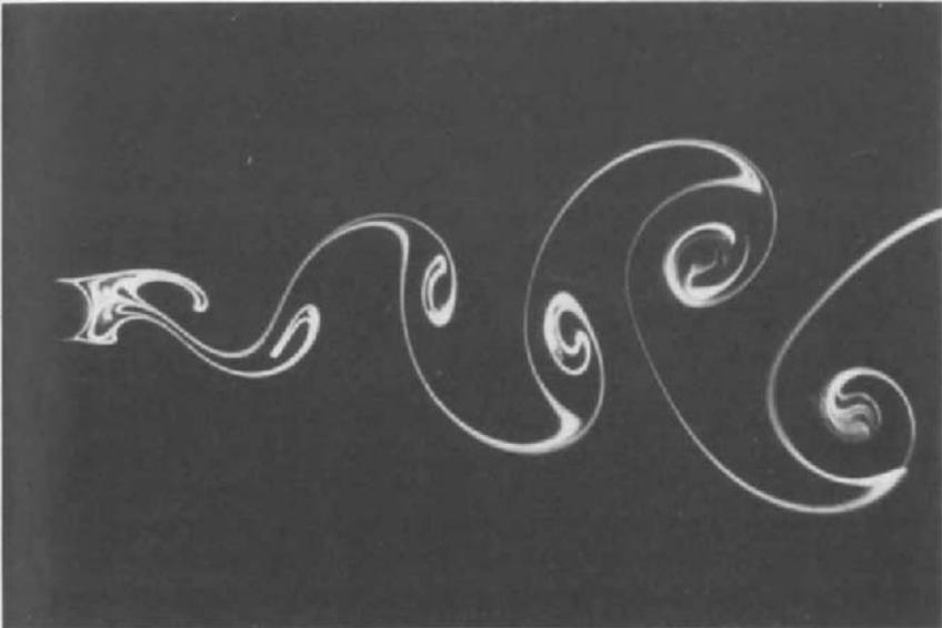
**Figure 1.12** A Karman vortex street behind a circular cylinder. Streaklines are shown by electrolytic precipitation in water. (Photograph by Sadatoshi Taneda; from “An Album of Fluid Motion,” assembled by M. Van Dyke and published in 1982 by Parabolic Press, Stanford, California.)
