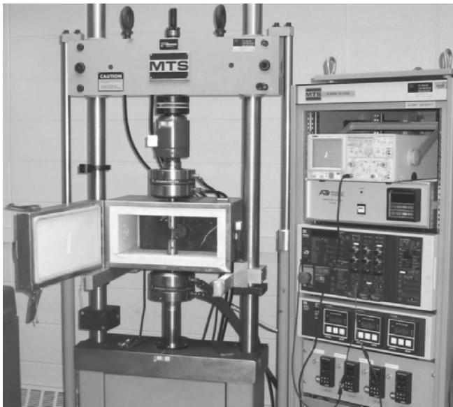
Fig. 5.6 Closed-loop servo-controlled hydraulic testing system.
