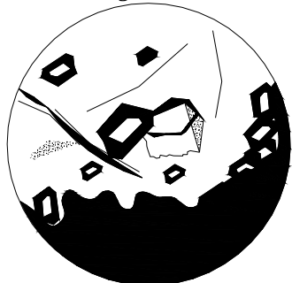
crystal and fissure inclusions in fire opal
