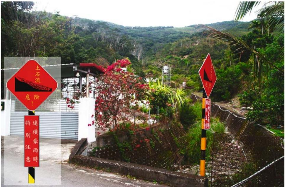
**Figure 21.19.** A debris-flow warning sign installed at the crossing of a road and a debris-flow-prone channel.
