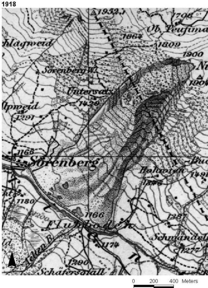
**Figure 24.6.** Topographic map, 1918. The open scars on either side of the mass and the freshly deposited material have been clearly delineated by the cartographer.
