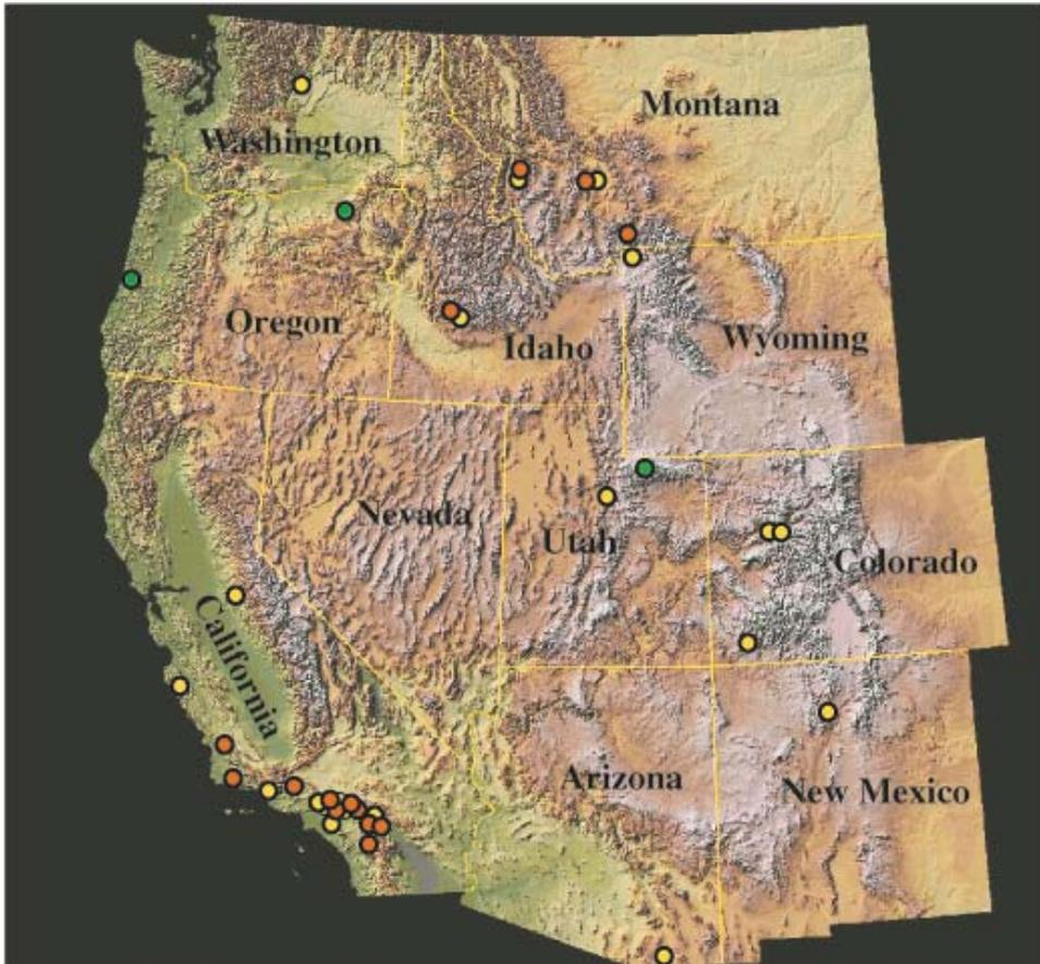
**Figure 15.2.** Map showing locations of documented fire-related debris-flow events in the western USA. Data for more than one basin exists at most locations. Yellow dots signify locations of basins for which data on either debris-flow volume or peak discharge exist (Gartner et al., 2004); both red and yellow dots show locations of debris-flow producing basins included in Gartner et al. (in press); green dots show additional debris-flow locations reported in the literature.
