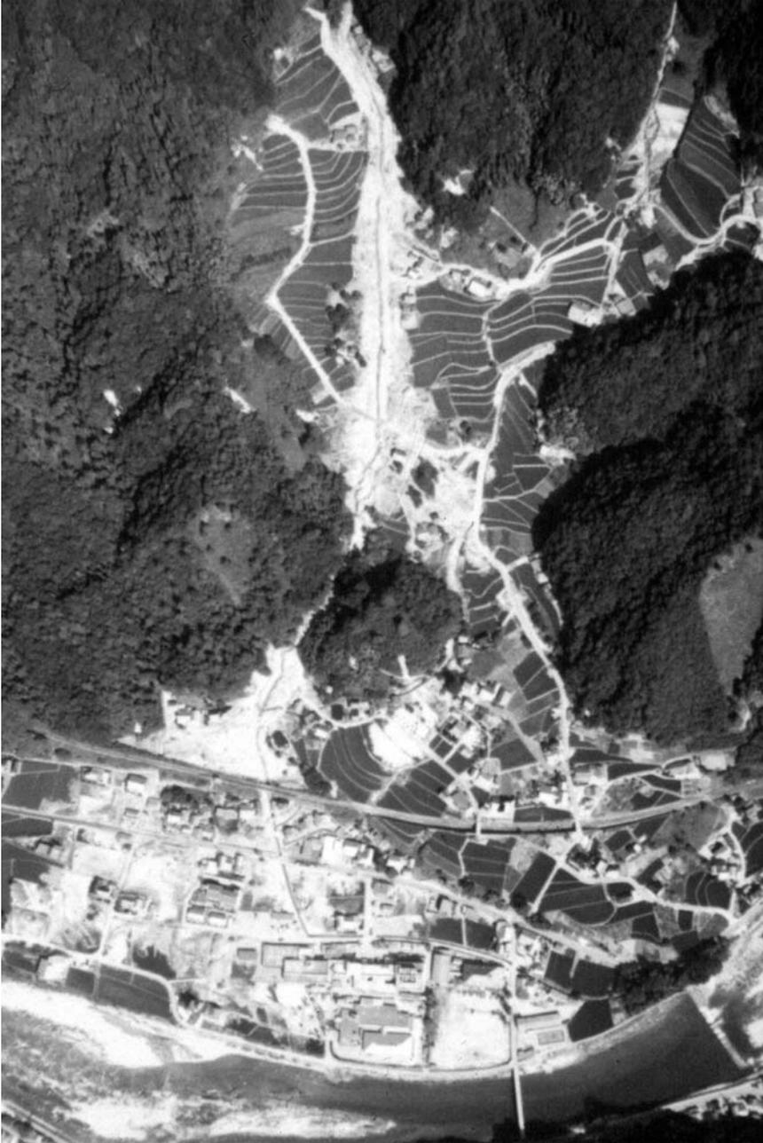
**Figure 1.3.** An aerial view of a debris fan in western Honshu Island, Japan, shortly after the impact of a debris flow, which destroyed several houses and killed 10 persons. Debris fans often constitute highly desirable development land, free of river flooding and steep land hazards, but at the price of exposure to debris flows.
