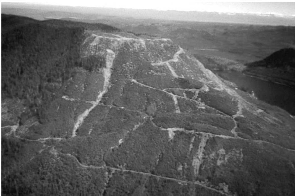
**Figure 2.4.** A group of debris avalanches triggered by logging and road construction on the west coast of Vancouver Island, Canada.
