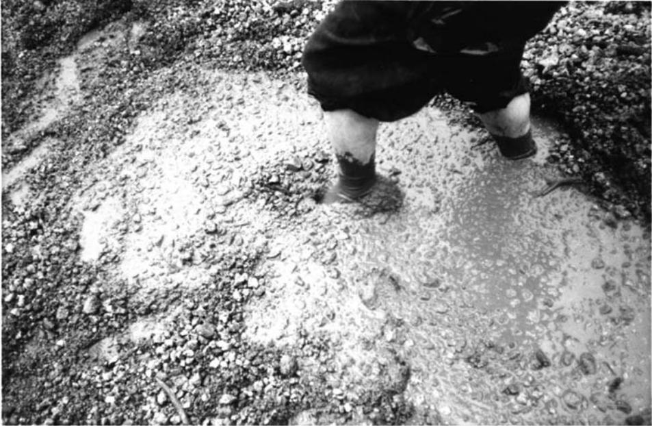
Figure 5.3. Torrent deposit liquefied by stamping some hours before the initiation of a debris flow.
