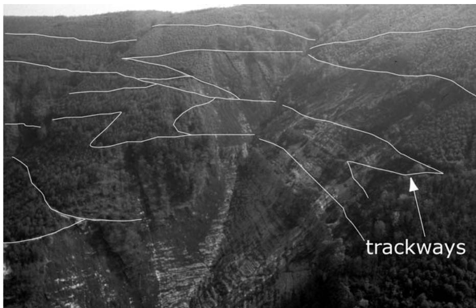
**Figure 19.21.** The slope involved by debris avalanches in the area of San Francisco gullies: note the remarkable link between initial failure and man-made cut. It is possible to observe the same area through photo-interpretation of the coupled images of Figure 19.7(b).
