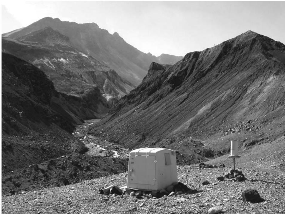
**Figure 12.2.** Loowit AFM station (Acoustic Flow Monitor, in housing centre) and precipitation gauge (on right), looking upstream towards Mount St. Helens' crater. Levee from a 1997 lahar is visible along the channel. Mount St. Helens' east crater wall is visible in the background.
