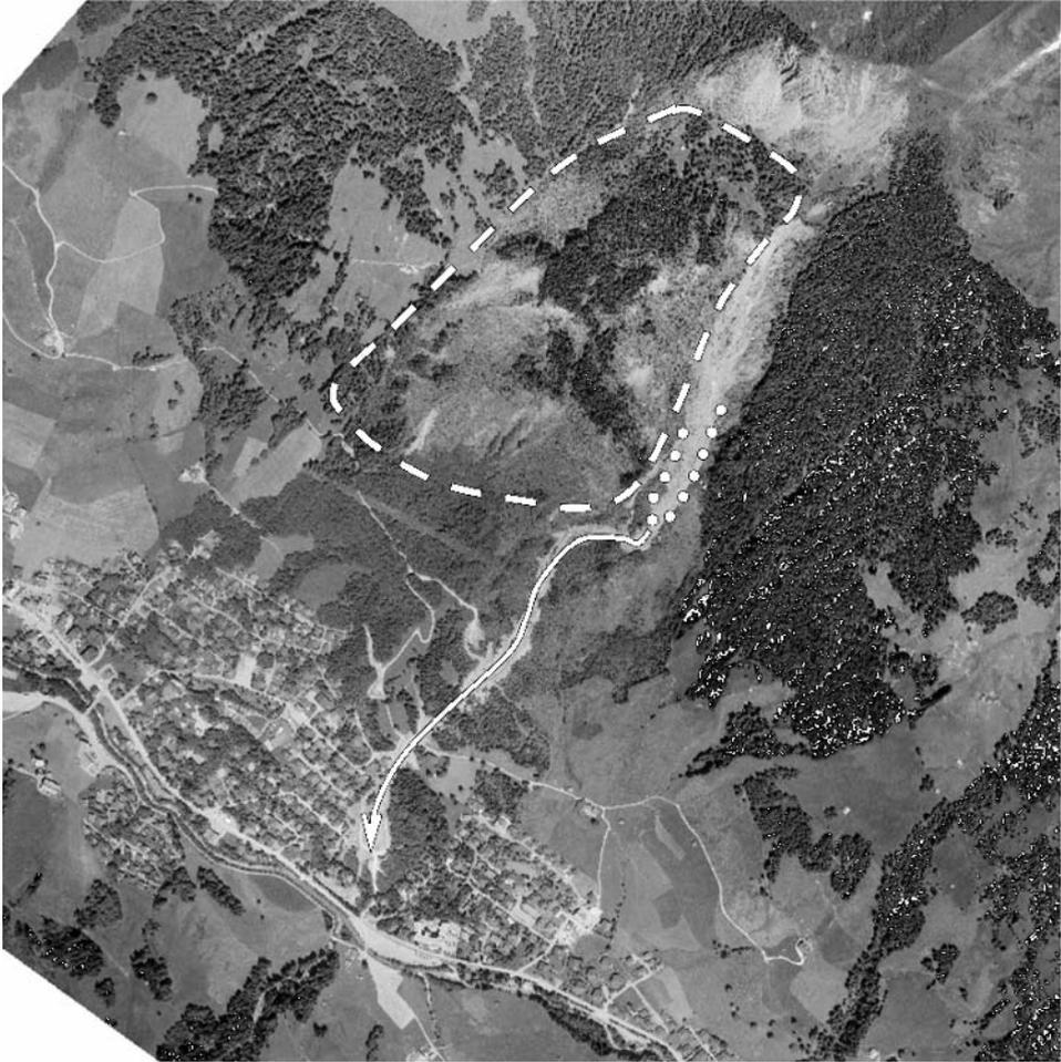
**Figure 24.4.** Aerial photograph of the landslide complex (July 1999). The deep-seated landslide (dashed line) has a volume of 15 million  $\text{m}^3$ . The dotted line marks the extent of the collapse and the subsequent flow (about 250,000  $\text{m}^3$ ). The black line indicates the flow path of the various debris flows which occurred in 1999.
