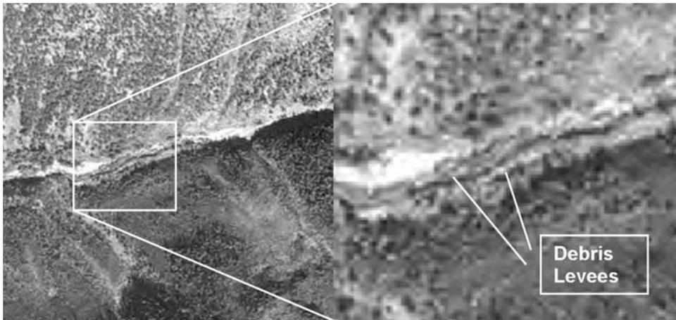
**Figure 11.4.** Trace of debris flow showing remnant levees in the Chetwynd area of British Columbia. Note that the spatial resolution of 1 m on the ground allows the recognition of debris flow levees.
