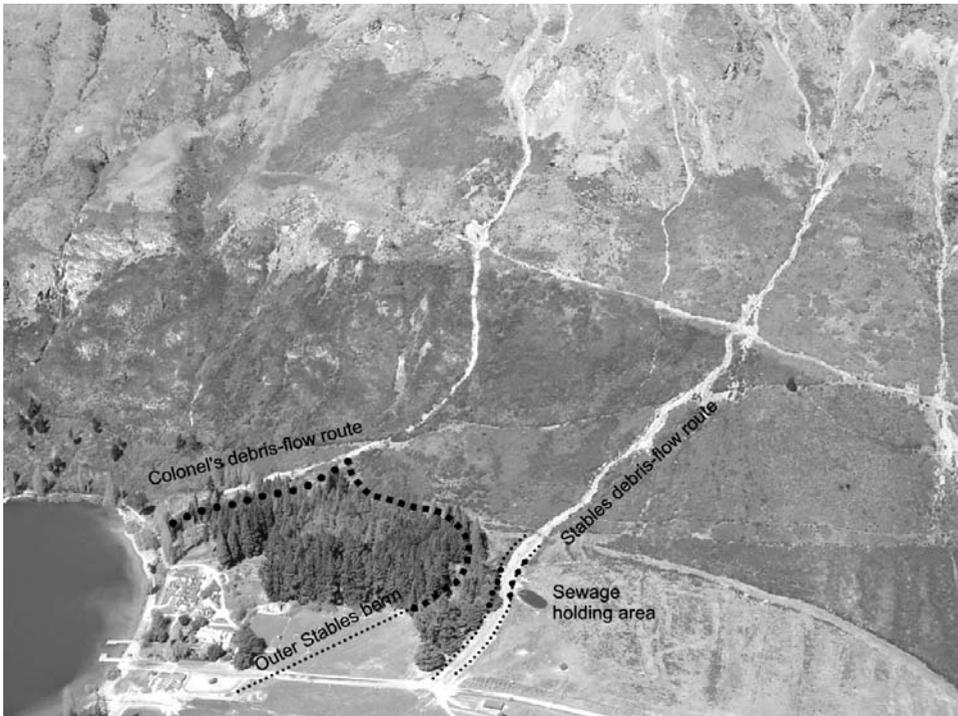
**Figure 25.2.** Aerial view of the Walter Peak debris flows of November 1999. The Colonel's debris flow on the left passes near to the Colonel's House. The Stables debris flow in the centre passed through the Walter Peak stables in November 1999.
