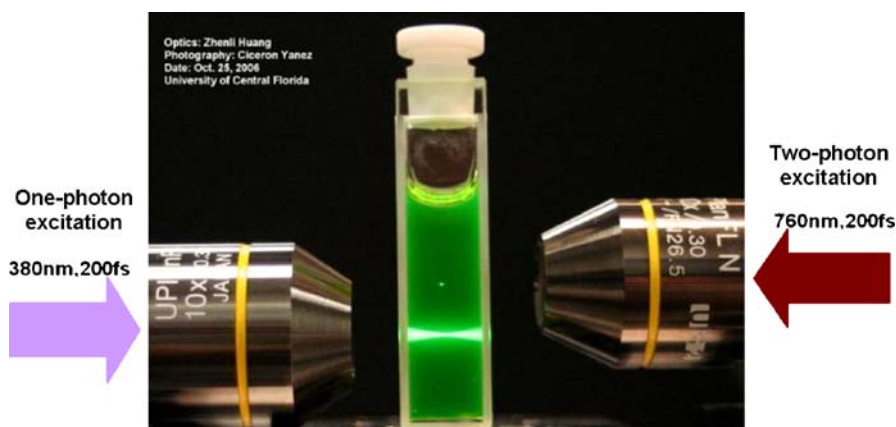
Fig. 1 Demonstration of the spatial selectivity of one-photon excitation ( left ) vs. two-photon excitation ( right ) in a fluorescein solution
