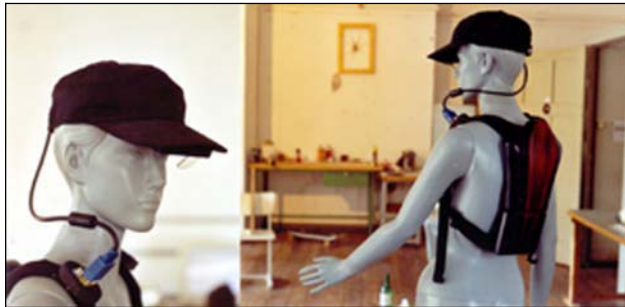
Figure 4 Volumetric model of the backpack housing with HMD plugged in at the collarbone connectors
