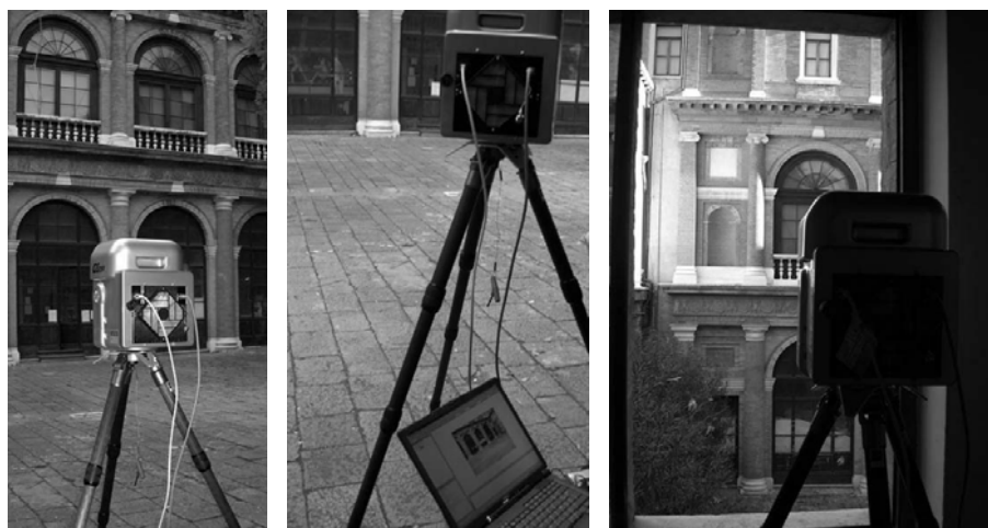
Figure 5-7 3D Laser scanning
