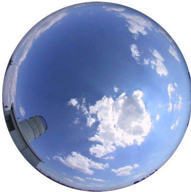
Figure 8 A sky image taken with a digital camera equipped with a fisheye lens
