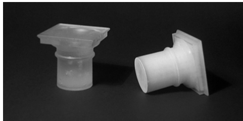
Figure 15 RP Techniques with resin for the construction of the Doric Capital
