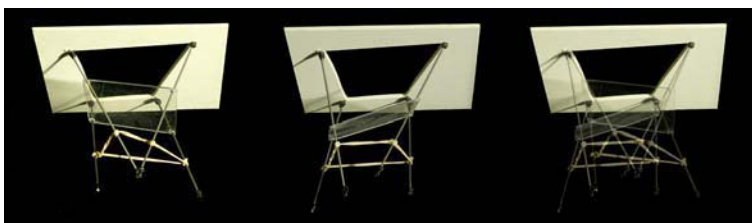
Figure 22 There are five sizes of glass proposed for the swimming pool, but many more variants for the actual opening sizes can be found using this analogue parametric model
