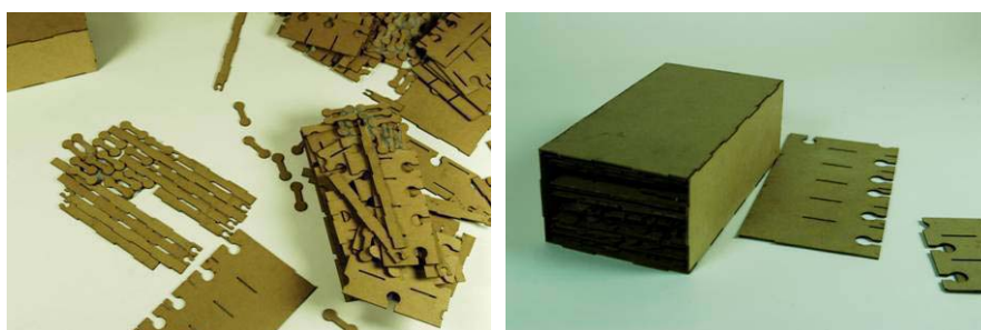
Figure 4 Left, photo of dog bones, studs, and wall panels with notches for dog bone connections cut of 1/16” cardboard stock simulating 3/4” plywood sheets Right, photo of panels, studs and dog bones in one packaged container
