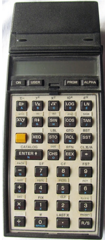
Fig. 7.1 The state of the art in mobile electronics circa 1982: Hewlett-Packard 41CV calculator with a 12 character display and memory of a few kilobytes
