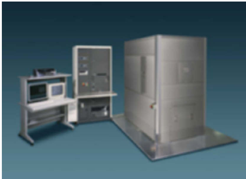
Figure 10.3 Top—A schematic representation of an Auger electron spectroscopy instrument. Bottom—A photograph of a commercial AES instrument (Physical Electronics).
