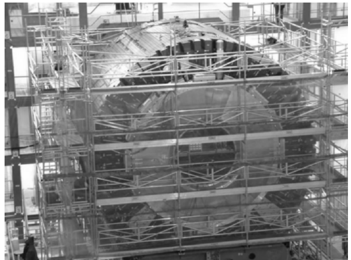
Fig. 6. The barrel calorimeter system in the underground cavern, with the cryostat containing the central solenoid and the barrel EM calorimeter, surrounded by the Tile Barrel Hadronic Calorimeter.
