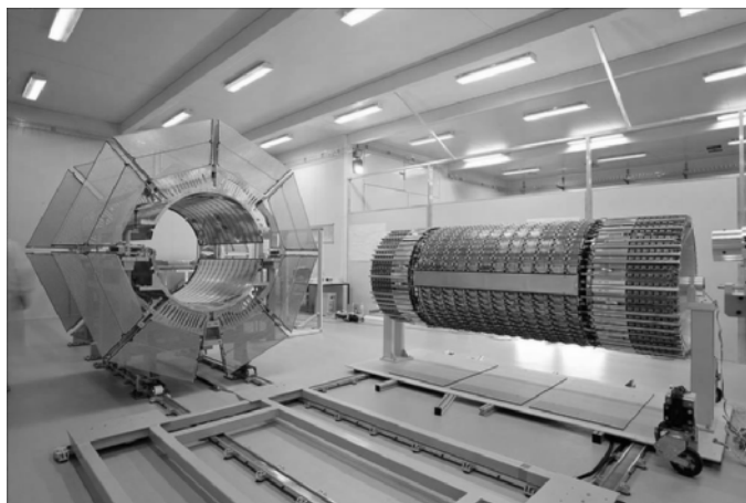
Fig. 4. The completed outer SCT barrel cylinder being installed in the thermal enclosure.
