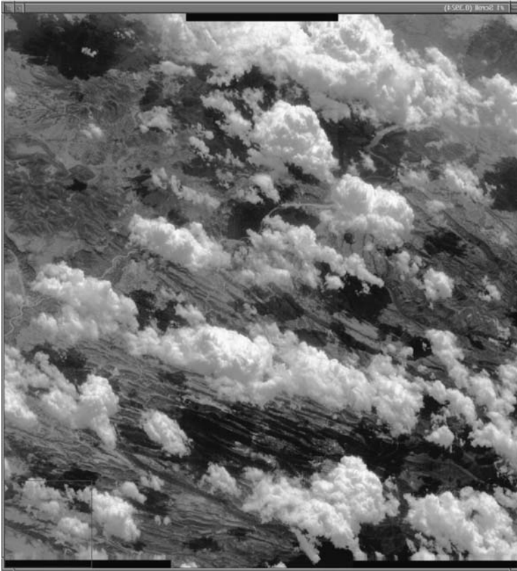
Fig. 3.17. Los Alamos (NM) scene with broken clouds captured with the Multispectral Thermal Imager (MTI) from a viewing angle of about 60°. This grey-scale image was produced from a true-color rendering of the scene based on 3 narrow channels at 484, 558, 650 nm. General characteristics of the MTI instrument and orbit are given by Weber et al. (1999). For a determination of mean optical thicknesses for three selected clouds with different outer sizes, see Davis (2002)
