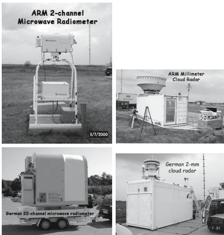
Fig. 1.9. Modern microwave ( left column ) and radar ( right column ) instruments for the study of 3D clouds in the US DOE's ARM Program ( top row ) and in Europe ( bottom row ). The ARM two-channel microwave radiometer stands a little over 2 m tall and is modified from a Radiometrics Corporation commercial product. The ARM cloud radar was developed by NOAA Environmental Research Labs in Boulder. Both ARM instruments point vertically and measure 2D time-height profiles. The European 2-mm-wavelength radar and 22-channel microwave radiometer scan together in lockstep, rapidly enough to capture the 3D structure of clouds; both are described at http://www.meteo.uni-bonn.de/projekte/4d-clouds/tools/
