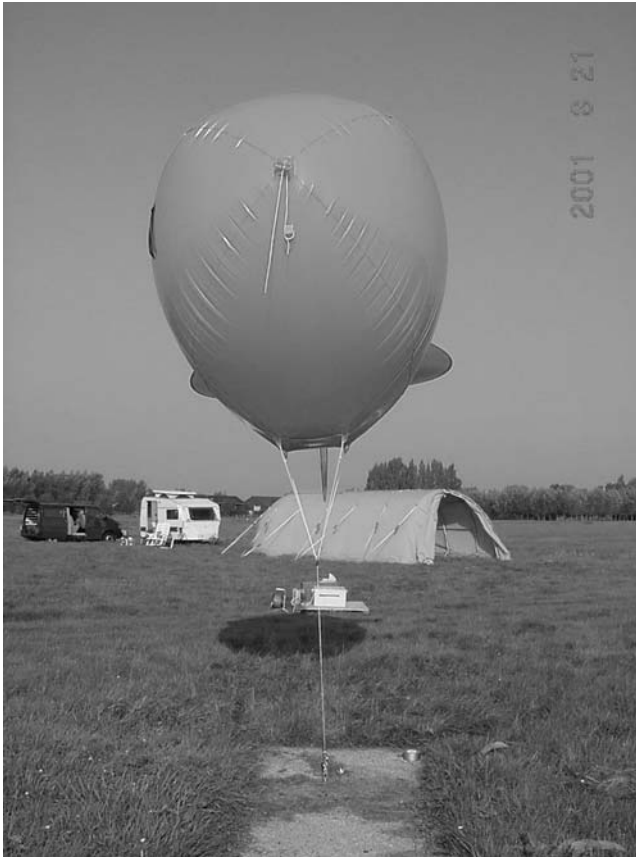
Fig. 1.10. Tethered balloon with cloud physics instrument payload developed by the University of Utrecht for the ASTEX field campaign in 1992, shown here participating in a 2003 field outing as part of the European 4D Clouds Project
