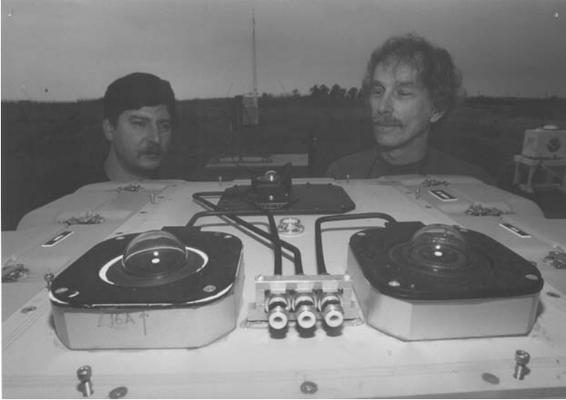
Fig. 1.19. Theoreticians Alexander Marshak ( left ) and the author puzzling over a strange alien object at the Oklahoma ARM site, which after considerable study they determined to be an “instrument”, in this case a set of pyroelectric broadband flux radiometers designed by Francisco Valero of Scripps. ARM brought many sallow-complexioned theoreticians out from behind their computer screens and into “the field” with considerable salutary effects on the cloud radiation subject
