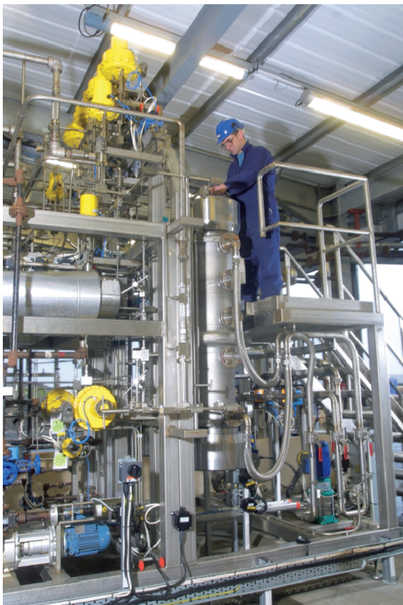
Figure 9. Photograph of the reactor array in the Thomas Swan and Co. SCF reactions plant.
