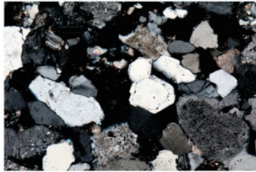
(c) 2684.5m, silica cementation
