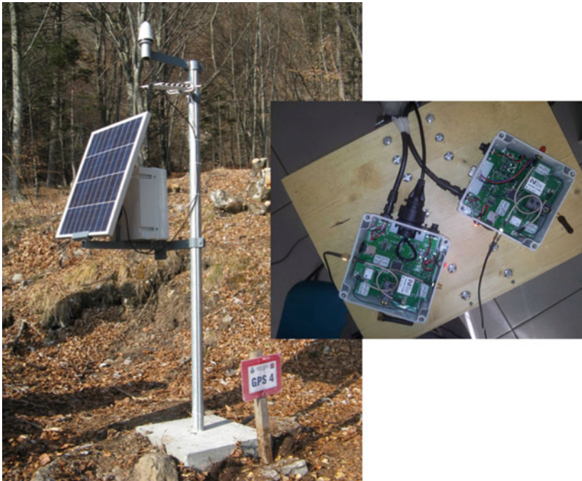
Fig. 7 SENDAS single frequency GNSS site for landslide monitoring
