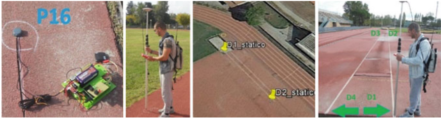
Fig. 12 u-blox and L1-L2 GNSS positioning on checkpoints and on flight strips simulation
