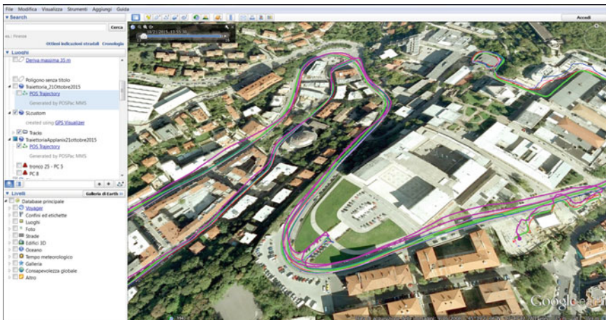
Fig. 8 A detail of the trajectories simultaneously surveyed using GeoSNav MMS ( green trajectory), GNSS Jupiter SL869 STD device ( red trajectory), customized GNSS Jupiter SL869 ( blue trajectory) and GNSS/GSM/GPRS GE910 ( purple trajectory) superimposed on ©Google Earth image
