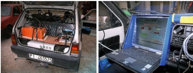
Fig. 3 Pisa MMS with instrumentation for air pollution monitoring
