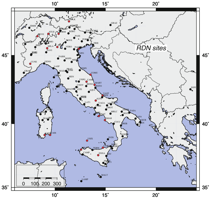
Fig. 2 The map shows all 99 official RDN sites. Red dots represent stations that are no longer sending data to the IGMI repository and black dots represent the 78 stations that are still operating and whose data are included in this work
