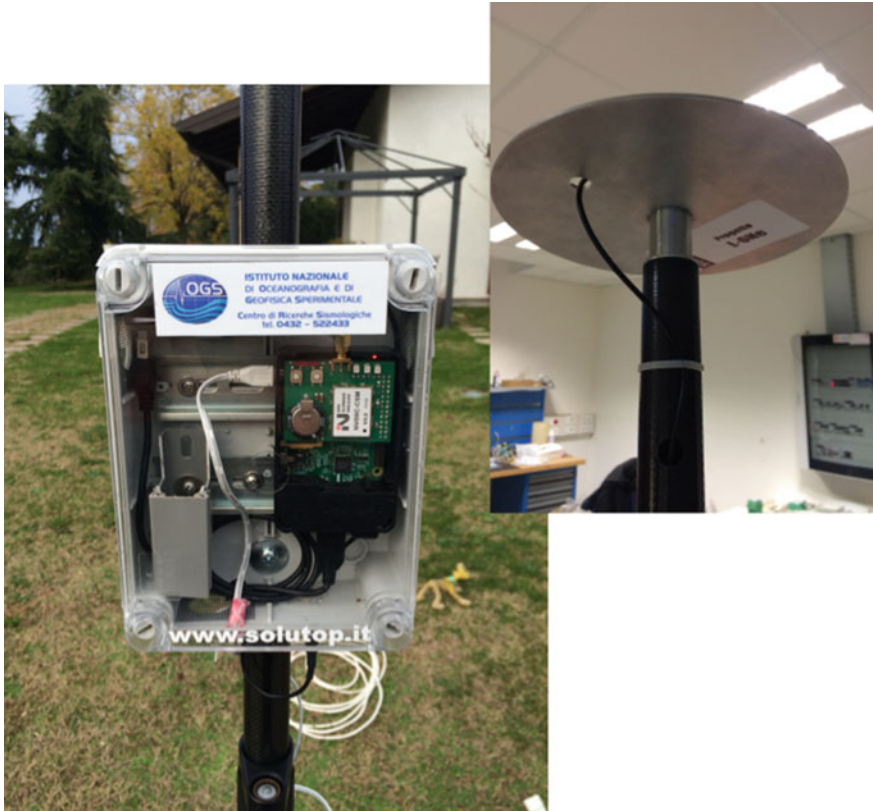
Fig. 8 LONE, single frequency GNSS device developed by OGS for RTK applications
