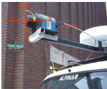
Fig. 7 The IBEO mono-axial Laser Scanner and an example of road cross section survey
