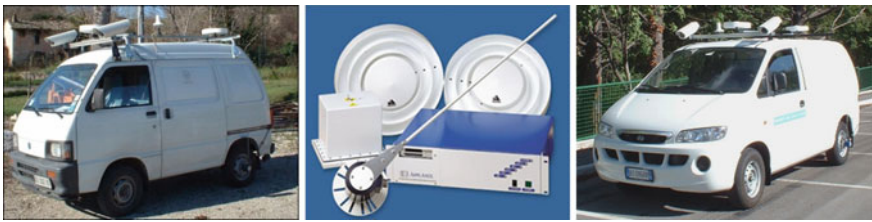
Fig. 4 The GIGI MMS ( left ), the Applanix POS-LV system ( middle ) and the MMS last version—GIGI One ( right )
