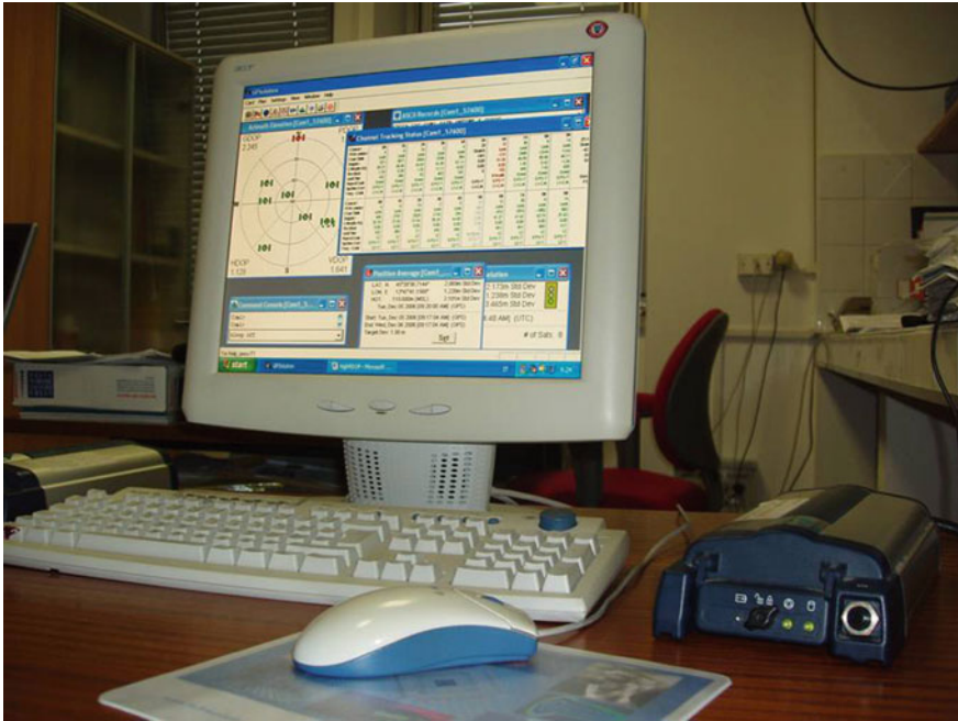
Fig. 4 The Experimental Data Server located at GeoSNav Lab, University of Trieste with the two Novatel MiLLennium GNSS (GPS + SBAS/EGNOS) receivers connected via two I/O ports. On the Server screen are shown the graphical interfaces and the command control and positioning status windows, showing the real-time SV plots, the channel tracking status with azimuth/zenith SV parameters, the signal frequencies, the SNR (Signal to Noise Ratio) parameters, and the tree-dimensional computed coordinates and accuracies
