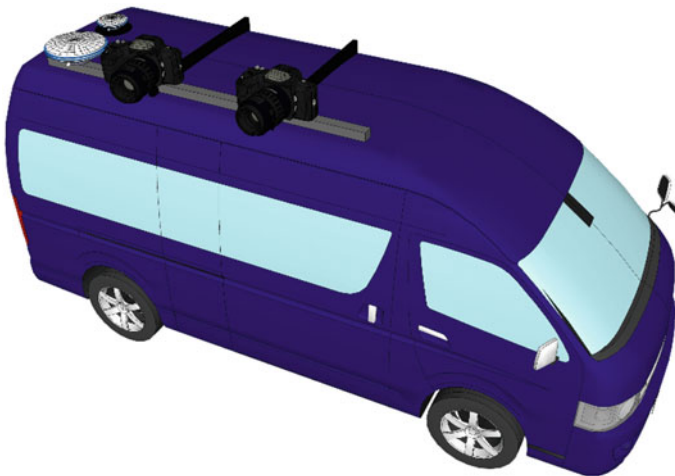
Fig. 1 The vehicle equipped with two cameras and two GNSS antennas used for the tests
