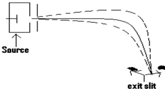
Fig. 13.25: A cylindrical electrostatic sector energy filter.
