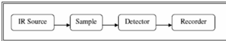
Fig. 13.48: Block diagram of IR analytical technique.
