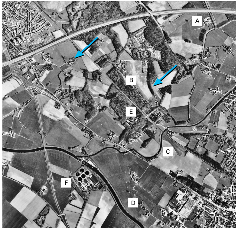
Figure 6.5. Aerial photo of an alluvial area covered with eolian sand (A) or river dunes (B). Minor (C) and main (D) streams and rivers are shown, as well as a well field (E) and a wastewater treatment plant (F). Doetinchem, The Netherlands (Topografische Dienst, 1997).
