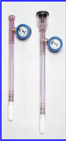
Figure 1.19. Tensiometers with porous cups and manometers to measure water pressure.
