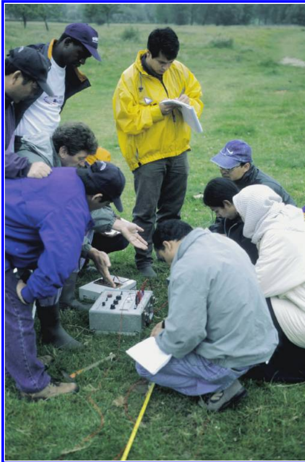
Figure 6.6. Execution of a geo-electrical measurement following the Schlumberger layout.
