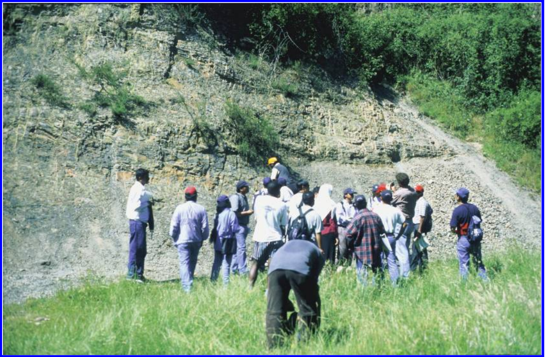
Figure 1.3. Hydrogeological assessments often start with rock observations. Here, students are inspecting slates and quartzites, dissected by joints and fractures.
