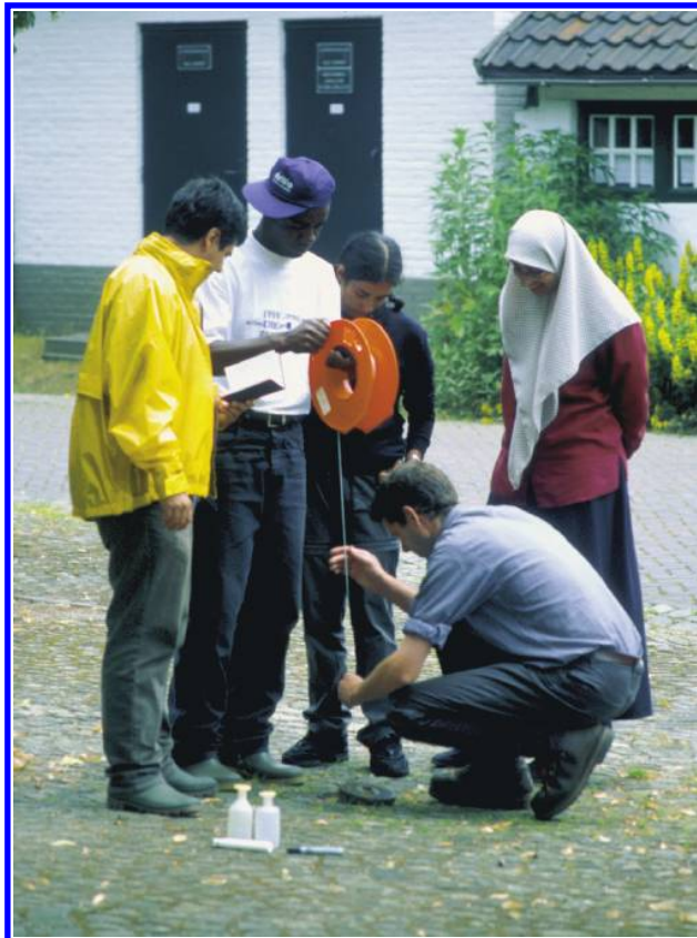
Figure 5.9. Water sampling with a simple device at a covered well in Limburg, The Netherlands.
