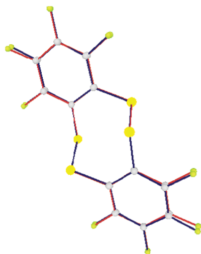
Figure 6-39. This complex polysulfide exhibits a nearly perfect fit, and indeed a perfect match of the torsional angles of the two disulfide chains although they are from polymorphic crystals – both monoclinic, P2_1/c and P2_1/a . BIBKUS and BIBKUS01 Ref. is [60]
