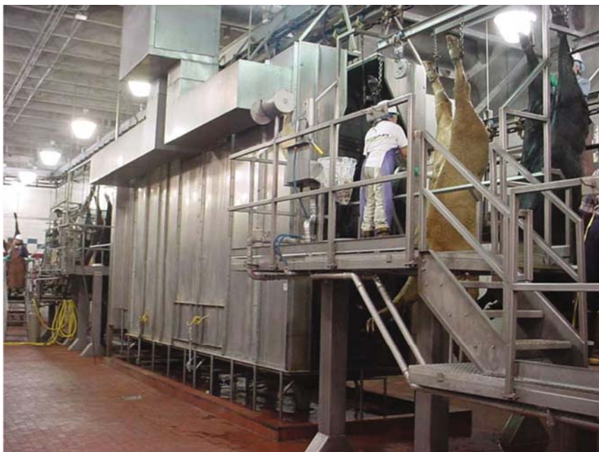
Fig. 13.2 Hide-on carcass wash and sanitizing assembly (Chad, 2004a)
