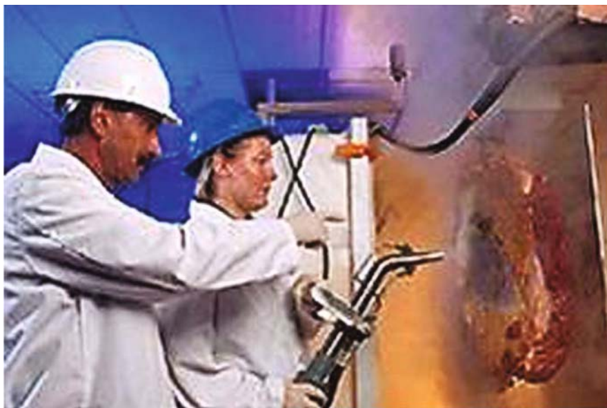
Fig. 13.5 Steam vacuuming of a section beef carcass (Weller, 2003)
