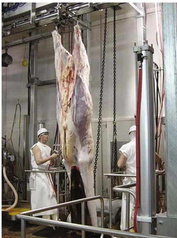
Fig. 13.3 Downward hide puller for the automated removal of hides (Milmech, 2004)
