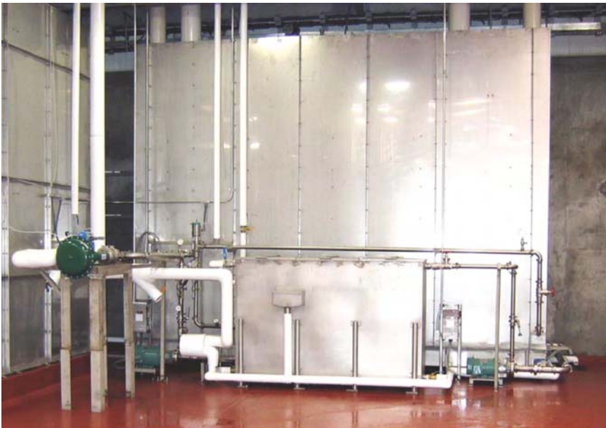
Fig. 13.7 Side view of carcass pasteurization system (Chad, 2004b)
