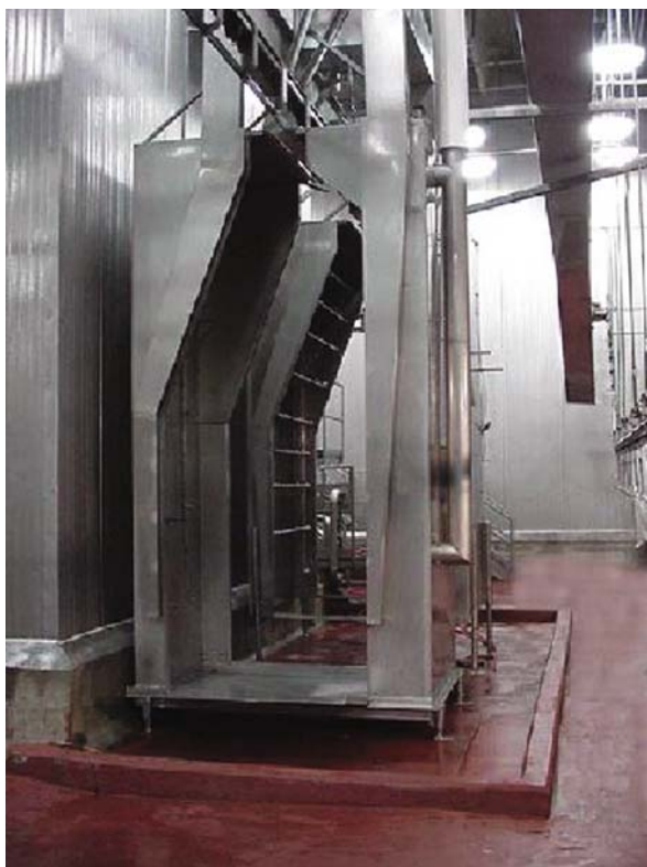
Fig. 13.4 Pre-evisceration carcass wash assembly and organic acid washer (Chad, 2004d)
