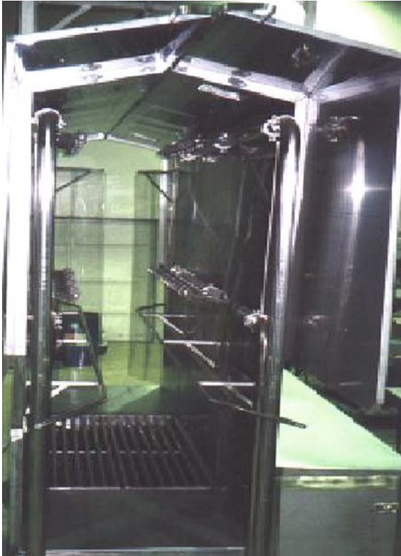
Fig. 13.8 Front view of carcass pasteurization system (Stanfos, 2004)
