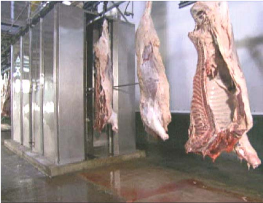
Fig. 13.6 Organic acid spray wash assembly (Chad, 2004c)
