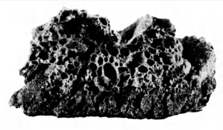
Figure 2. Slagging deposit showing segregated development.
