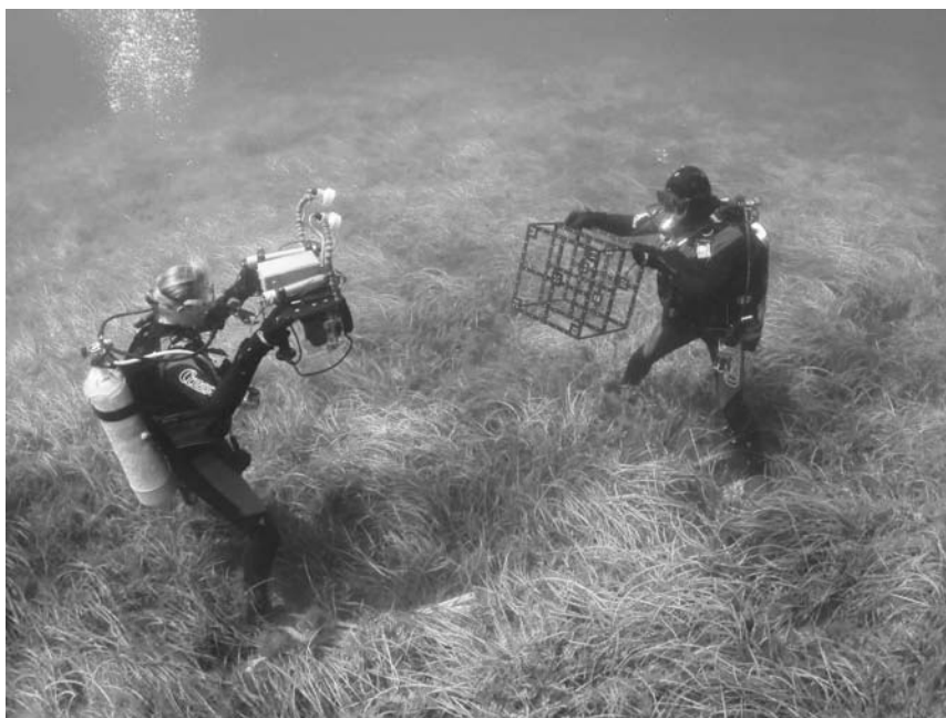
Figure 6 Underwater photography of a calibration fixture. (Courtesy D.A. Abdo.)
